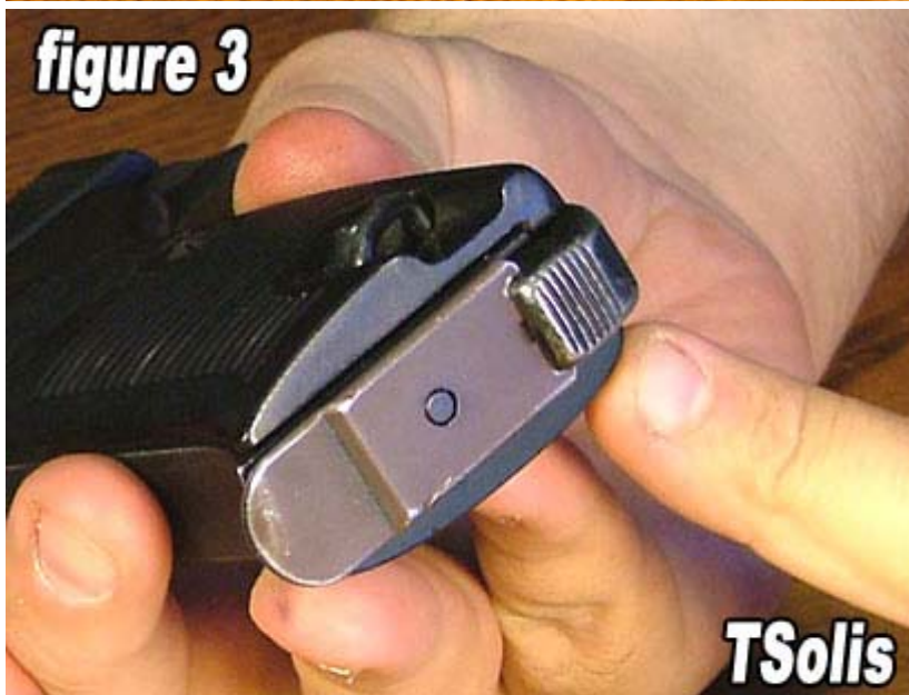
3) Figure 3 shown the P.38 pistol's magazine release.
