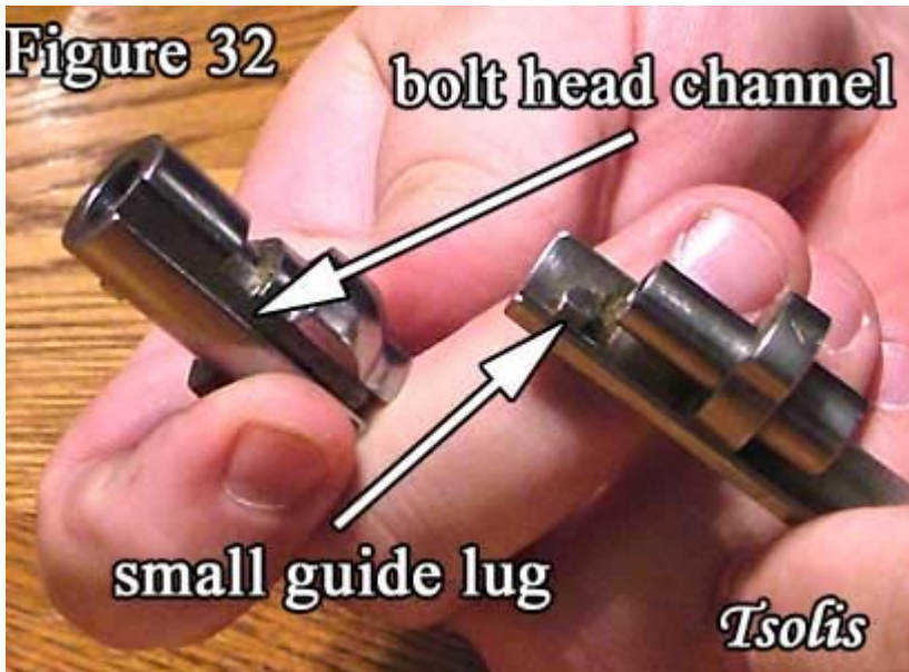
32) Figure 32 shows the channel in the bolt head on the left and the small guide lug on the connecting bar on the right.
