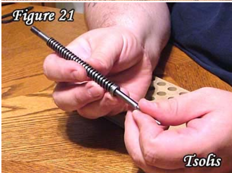
21) Return the firing pin spring to the firing pin.
