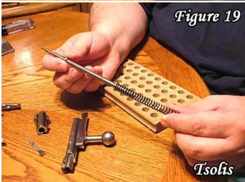
19) Remove the firing pin spring from the firing pin.
