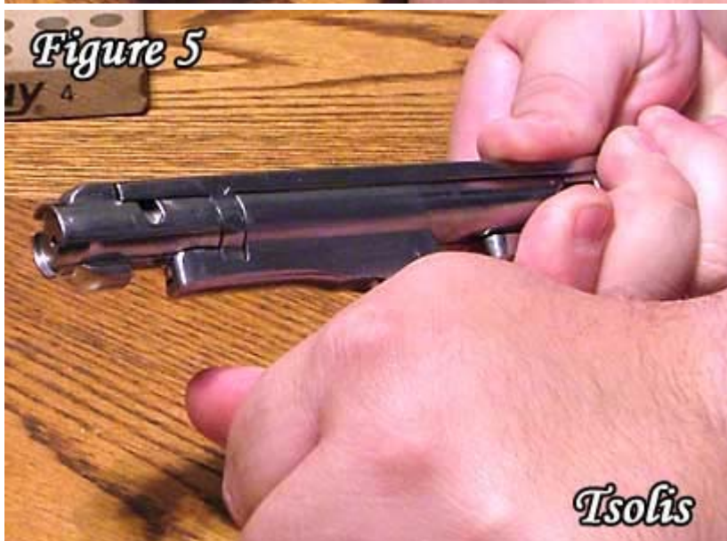
5) Rotate the cocking piece and connecting bar counter-clockwise 1/4 turn.
