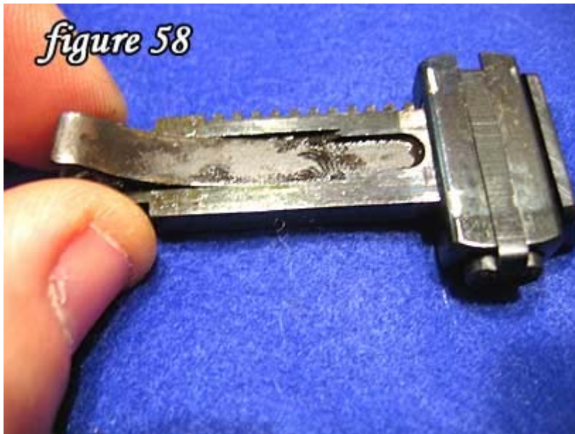
58) Slide the flat spring into its slot on the rear sight.
