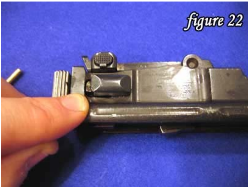
22) Figure 22 shows the bolt retainer released.
