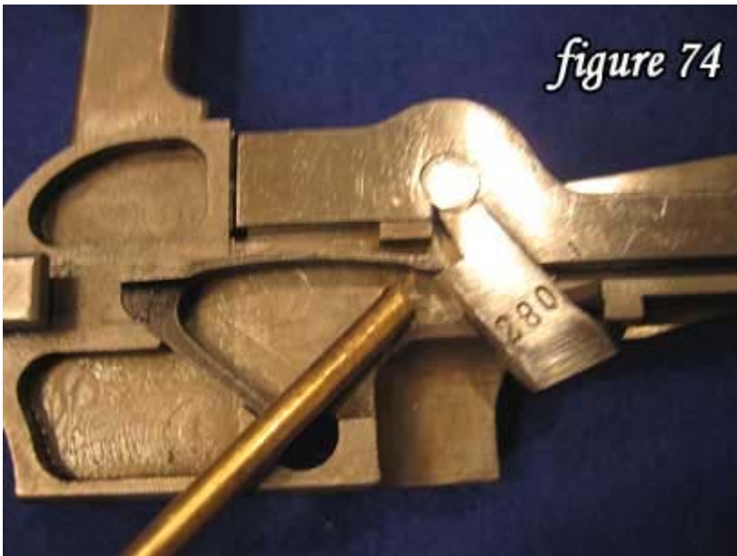
74) Note how the spring locks the disconnector into place.
