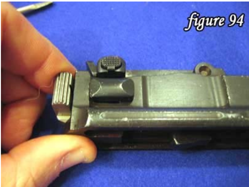
94) Note how the bolt stop seats flush up against the back of the barrel extension.
