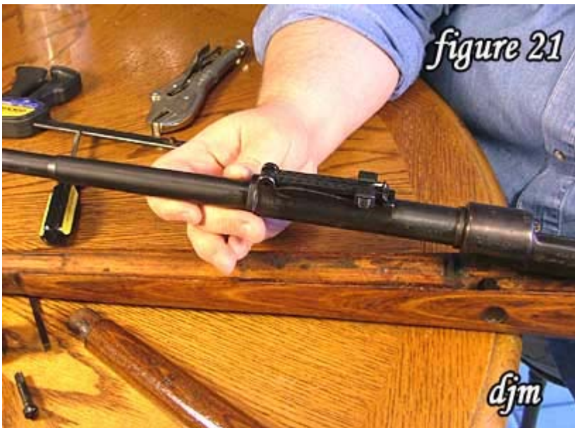
21) Lift the barreled receiver from the rifle stock.
