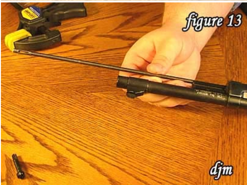
13) Remove the cleaning rod.
