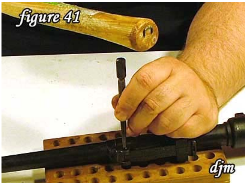
41) Tap the rear sight pin in place.
