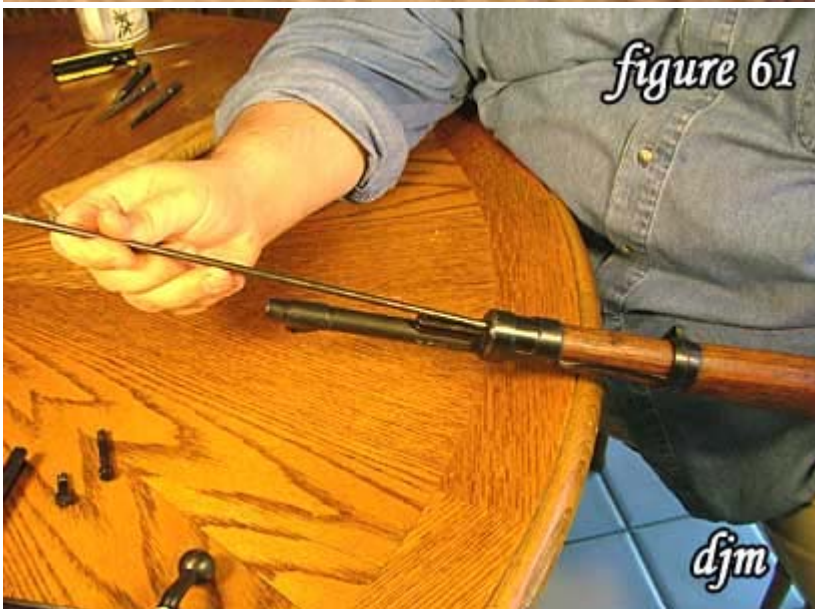
61) Slide the cleaning rod into the carbine.
