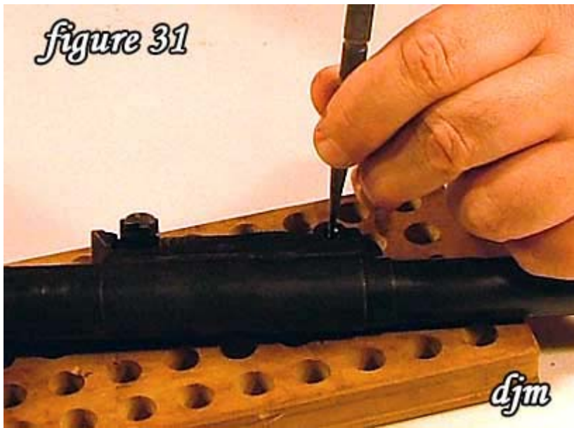
31) Using a punch, tap out the rear sight pin.
