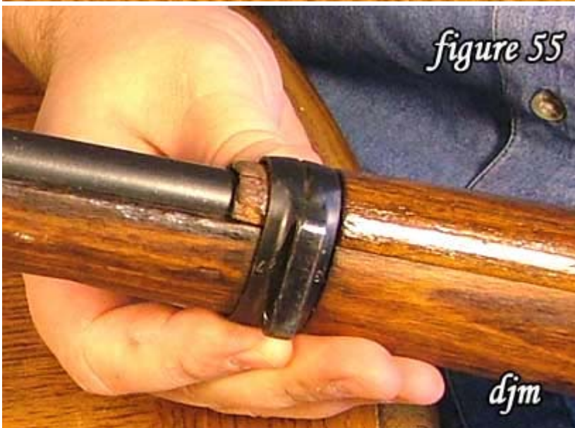
55) Slide the lower band into place.
