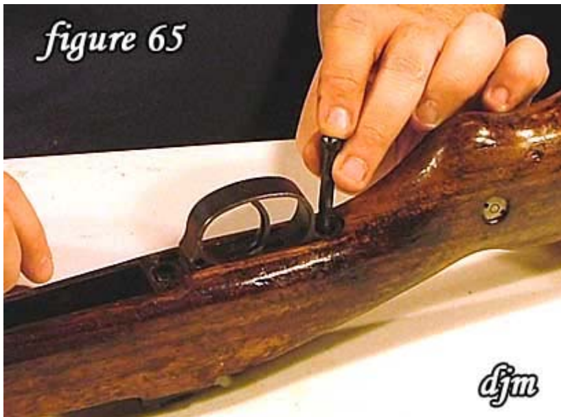
65) Install the rear guard screw.
