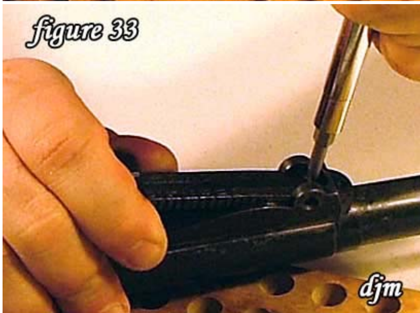
33) Place a flat blade screw driver in the indentation at the forward part of the rear sight leaf.
