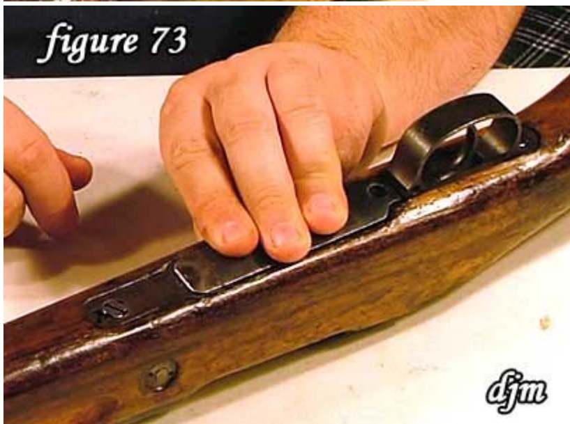
73) Hook the front of the magazine floor plate into the groove in the front of the magazine well and then lock the magazine floor plate into place.
