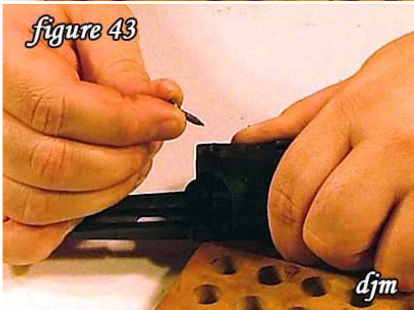
43) Install the bolt stop screw.
