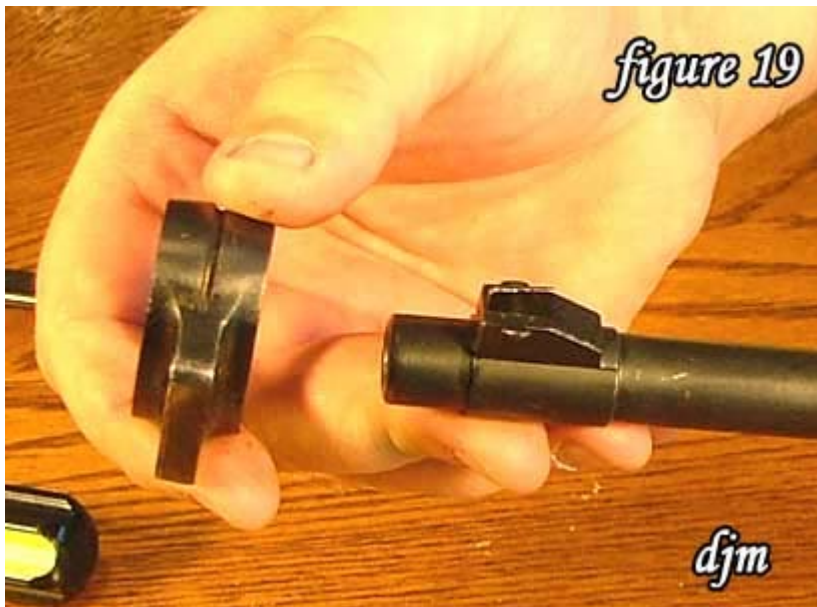
19) Remove the rear band.
