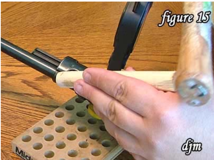
15) Tap the forward band forward.
