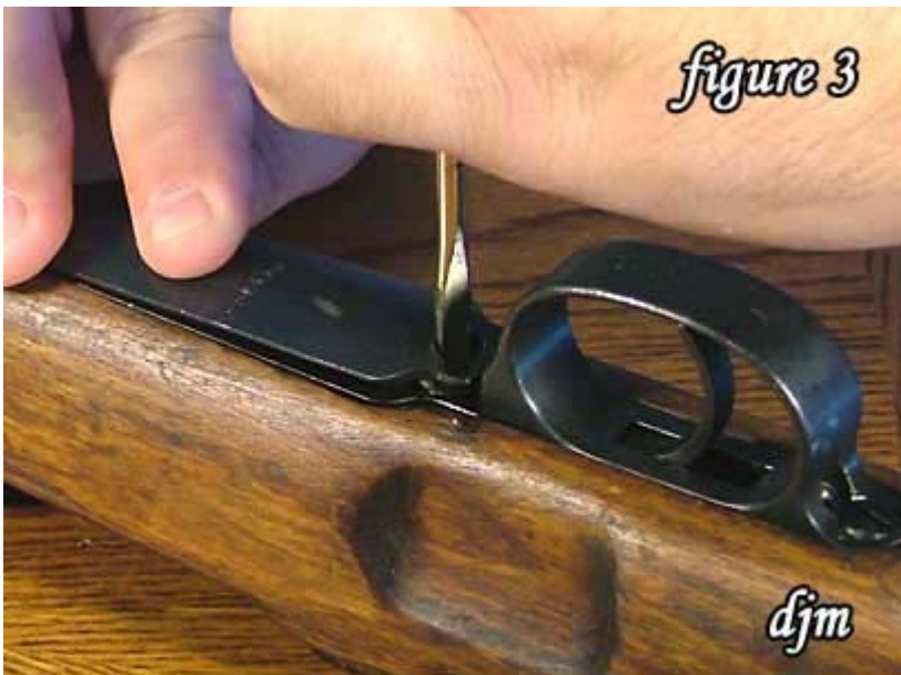
3) Depress the magazine floor plate catch.
