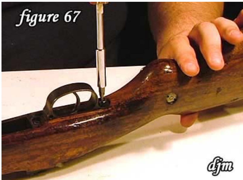
67) Tighten the rear guard screw partially.
