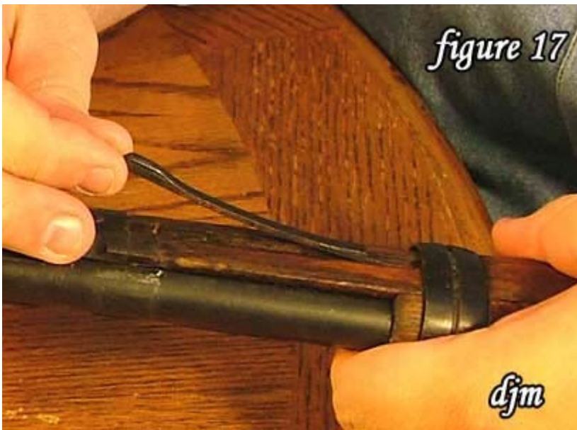
17) Remove the band spring.
