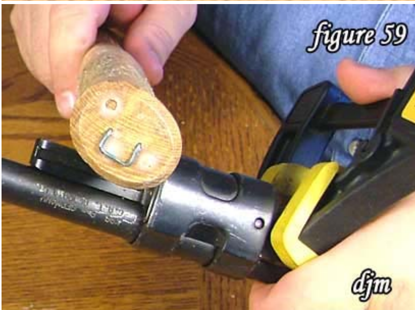
59) Tap the forward band into place. Using a hickory hammer handle is a great non-marring tool for tapping parts into place.
