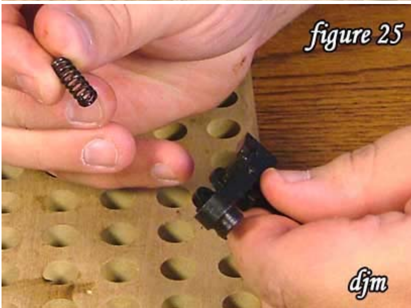
25) Remove the sear spring from the sear.
