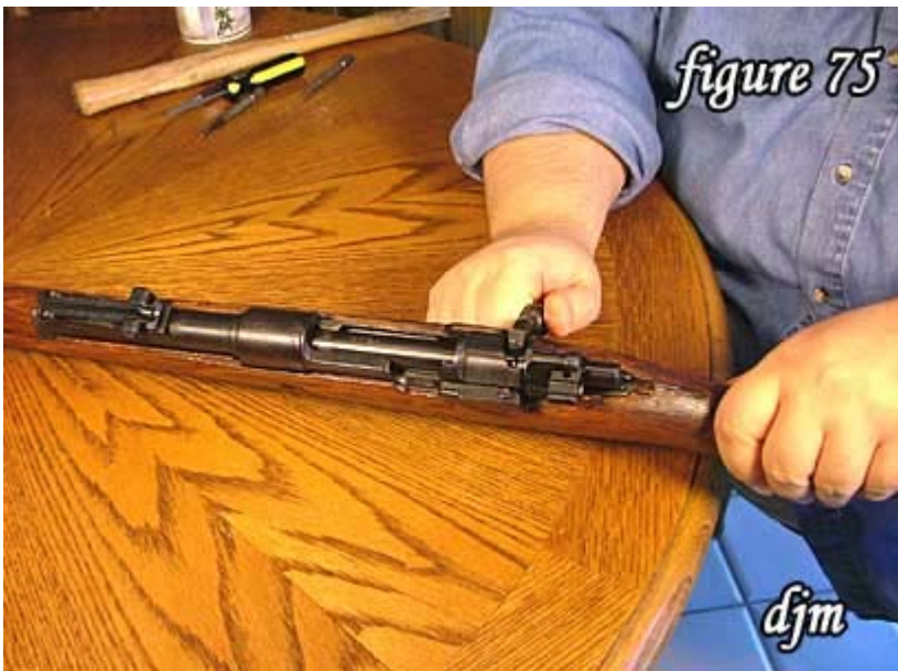
75) Close the bolt and you are finished reassembling the 98k carbine.
