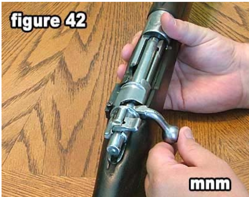
42) Move safety from middle position and you are finished disassembling and reassembling the Mauser bolt.
