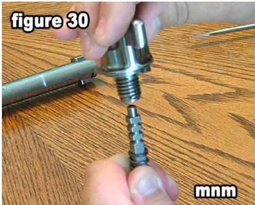
30) Place the bolt sleeve over the rear of the firing pin (as shown in figure 30) and place the tip of the firing pin pointing down into a block of wood.
