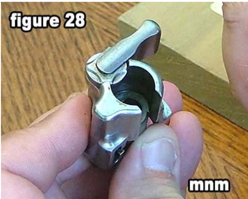
28) Figure 28 shows the safety properly installed.
