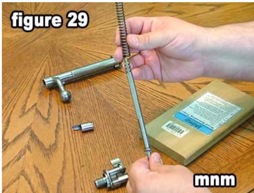
29) Slide the main spring onto the rear of the firing pin.
