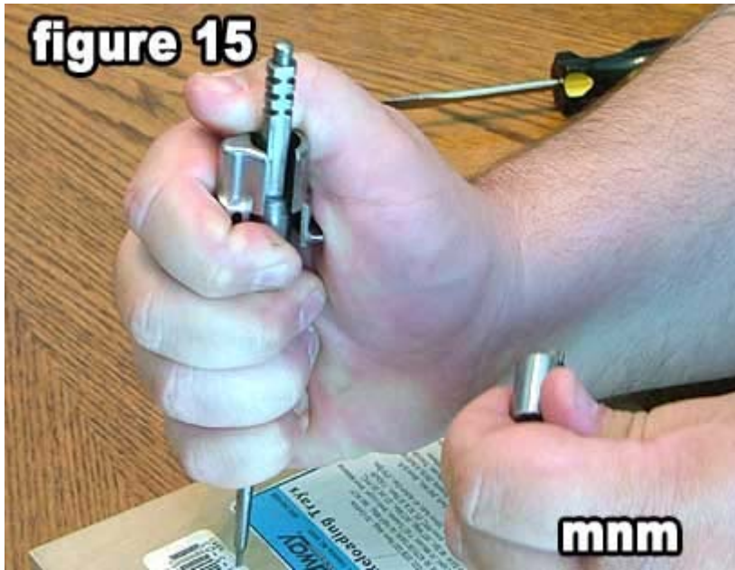
15) Remove cocking sleeve and set aside.
