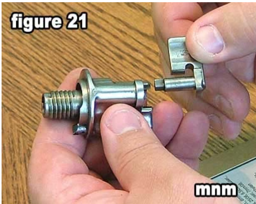
21) Remove the safety lever and set aside.
