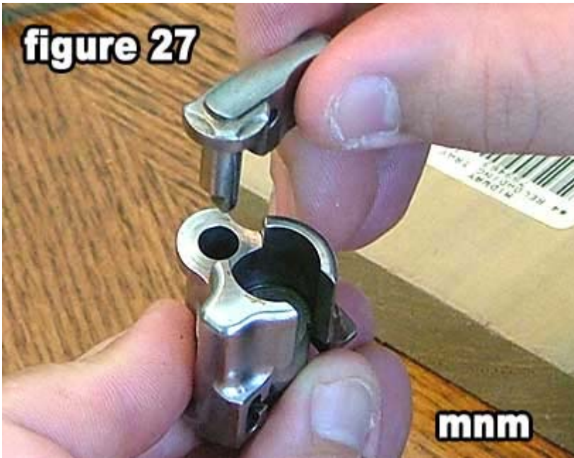
27) Insert safety into rear of bolt sleeve as shown in figure 27.
