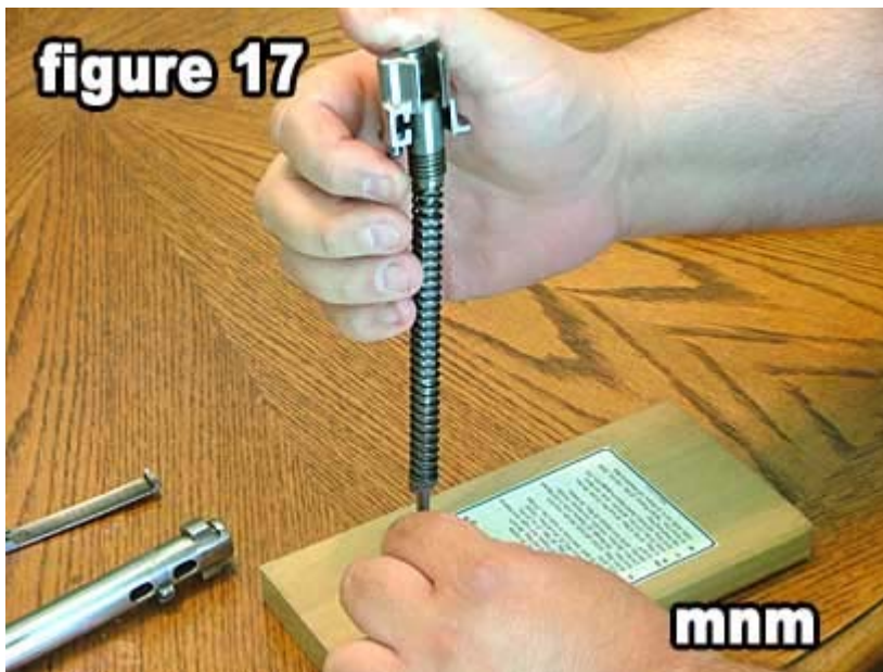
17) Allow main spring to fully expand as shown in Figure 17.
