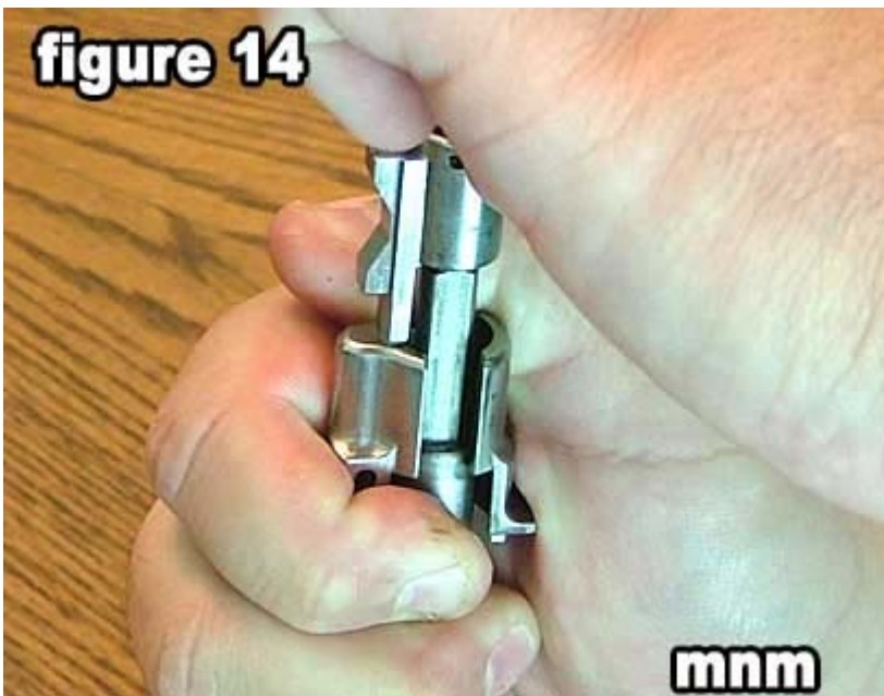
14) Turn cocking sleeve 1/4 turn in either direction.
