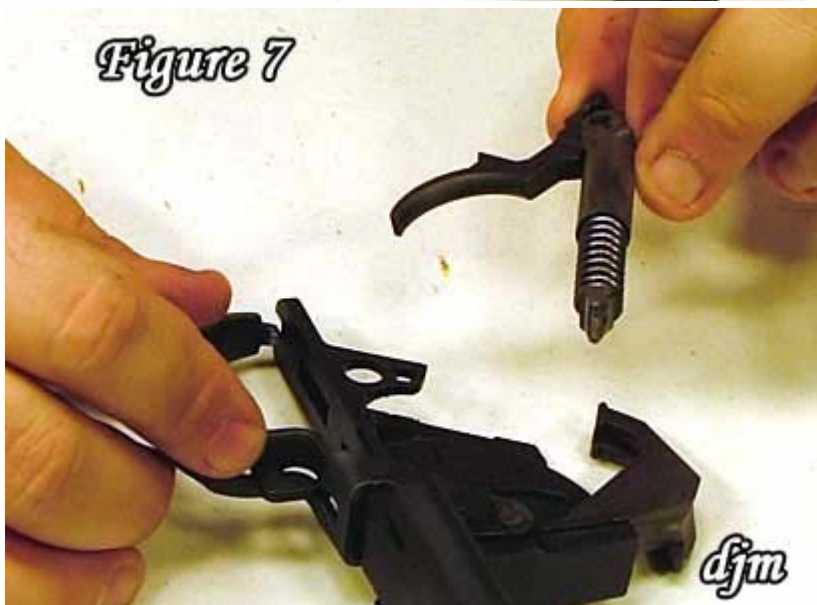
7) Remove the trigger, sear, spring, hammer spring housing, and plunger.
