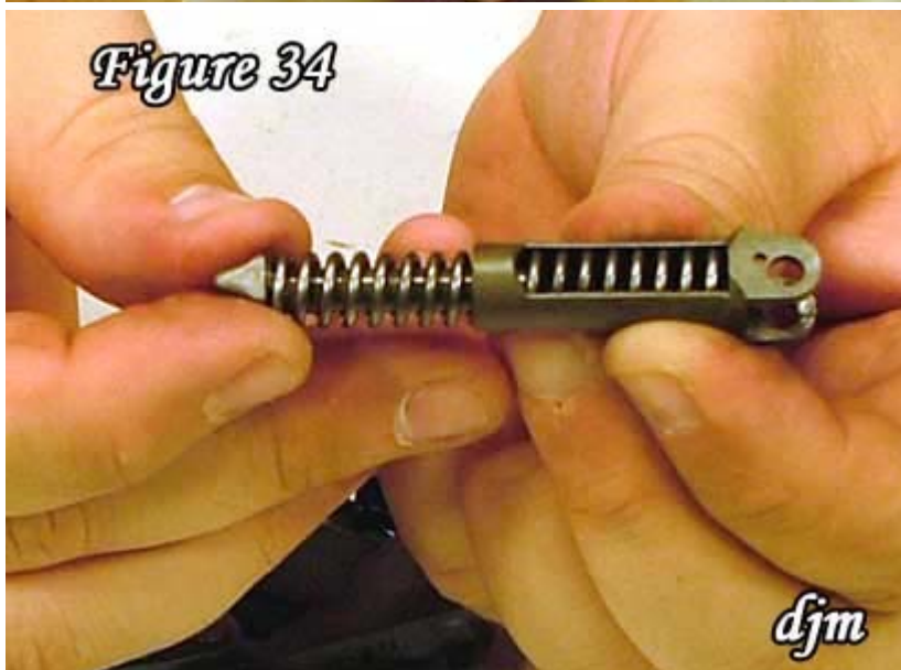
34) Insert the spring and plunger into the hammer spring housing.
