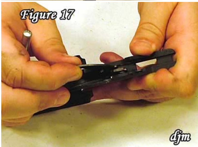
17) Pull the safety away from the trigger housing.
