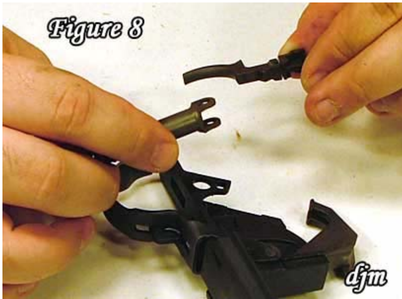
8) Separate the trigger, sear from the spring, hammer spring housing, and plunger.
