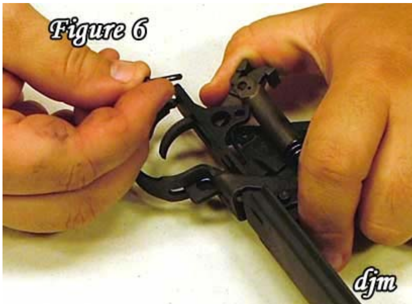
6) Allow the hammer spring to expand fully.
