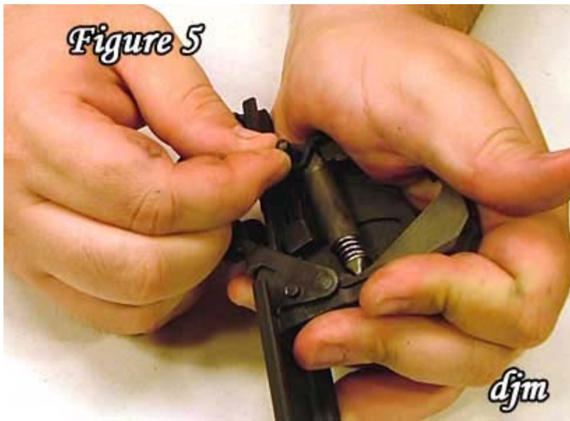
5) While holding the trigger and sear in place with the palm of your hand remove the trigger pin.
