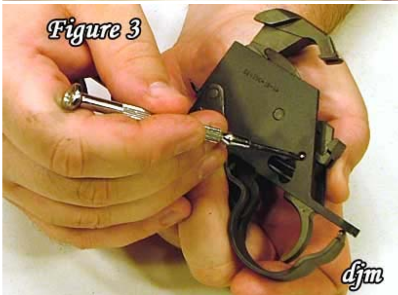
3) Figure 3 show the left side of the trigger pin.
