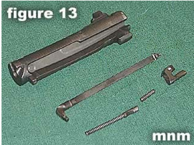
13) Figure 13 shows the disassembled bolt Assembly.
