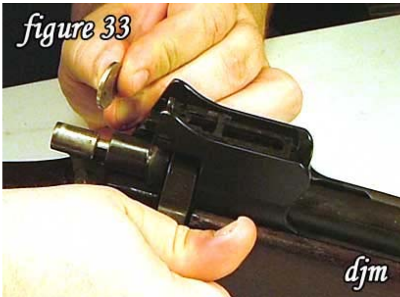
33) Apply forward pressure on the bolt handle and remove the coin from gap.
