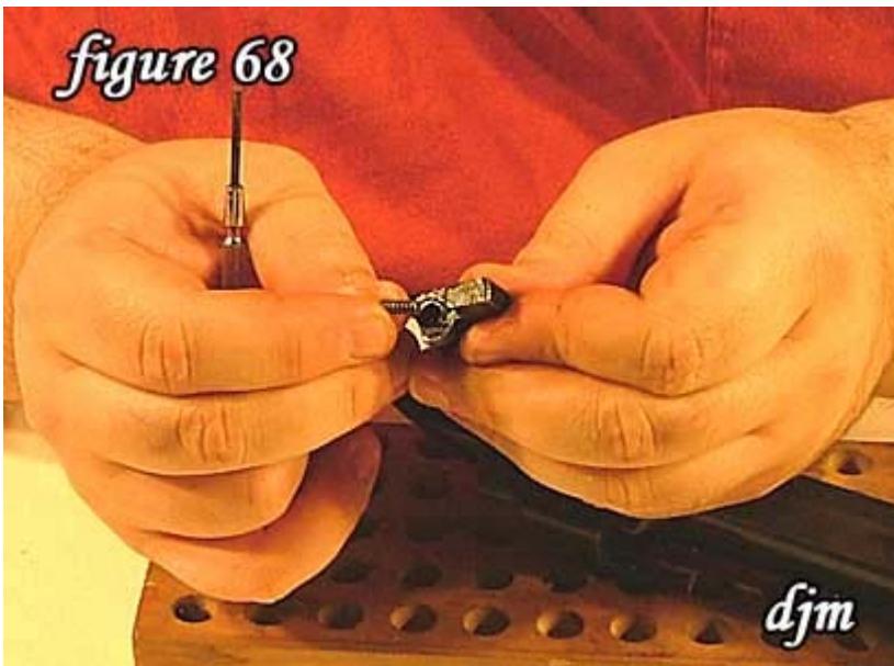
68) Insert plunger spring into cut-off.
