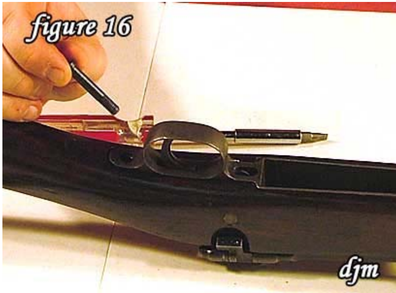
16) Remove the rear guard screw.
