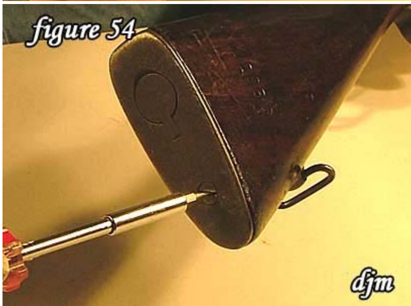
54) Tighten the lower butt plate screw.
