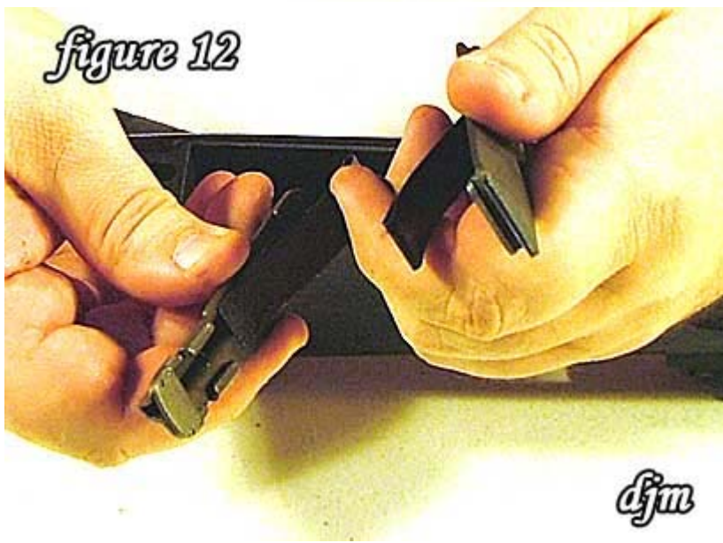
12) Separate follower from magazine spring.
