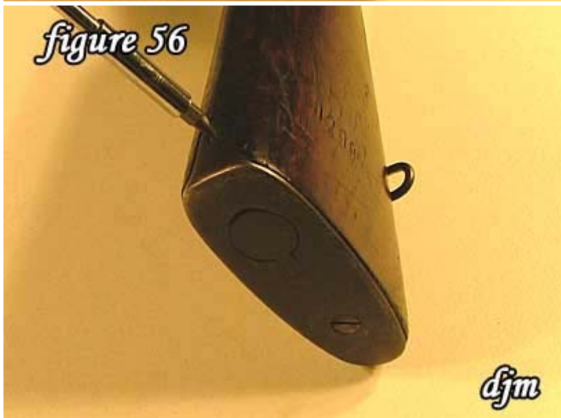
56) Tighten the upper butt plate screw.
