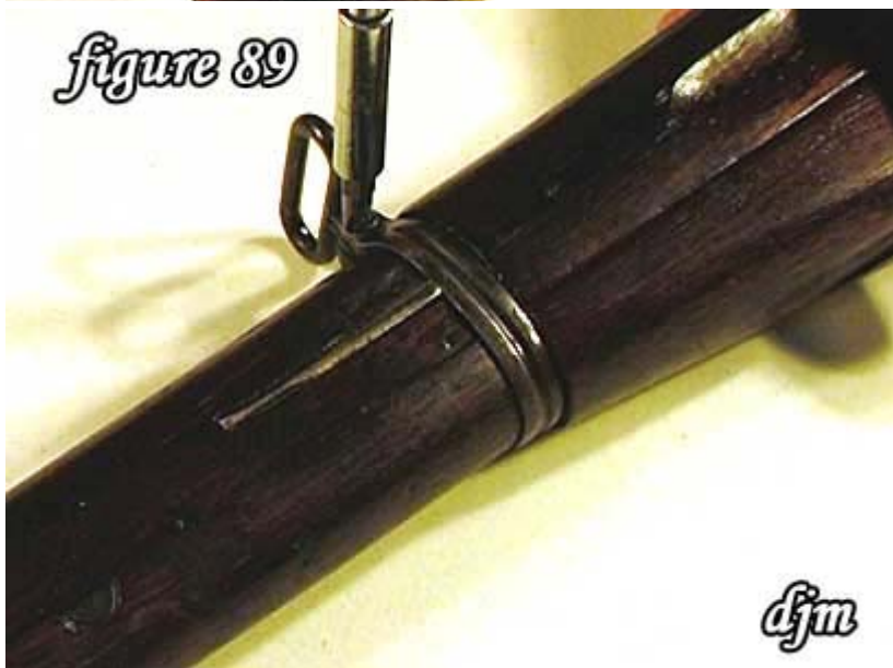
89) Tighten the rear lower band screw.
