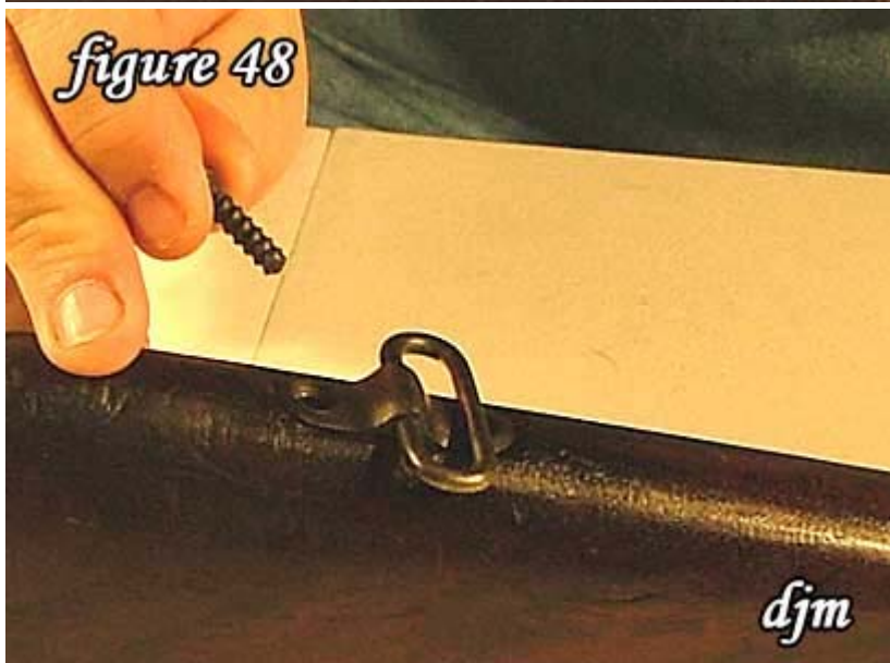
48) Replace the rear rear swivel screw.
