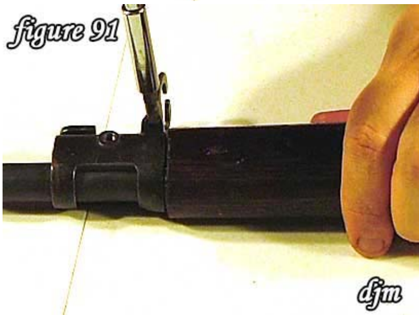
91) Tighten the stacking swivel screw.
