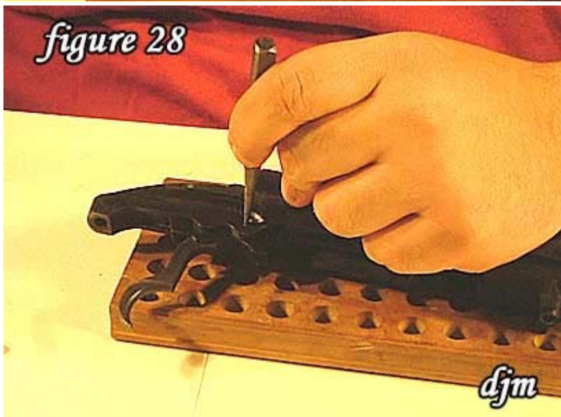
28) Remove the sear pin by driving it out with a punch.
