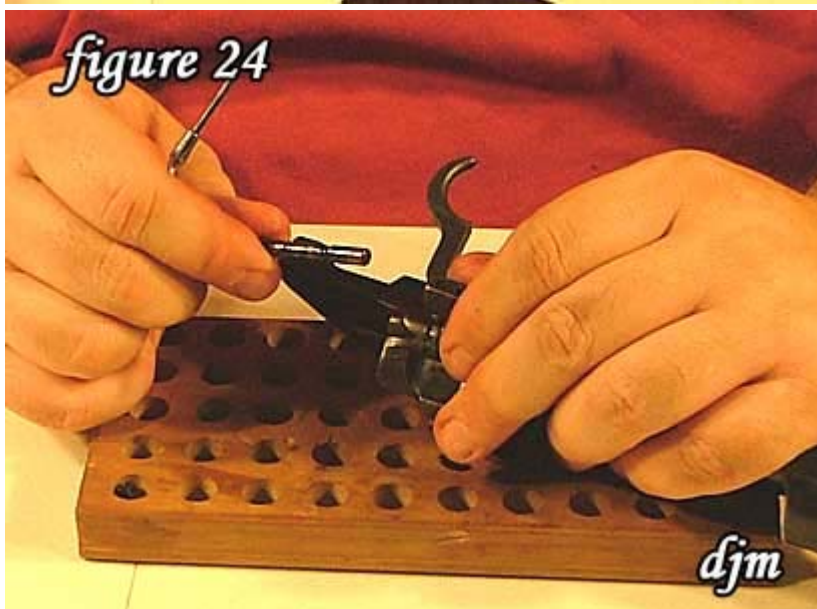
24) Remove the cut-off spindle.
