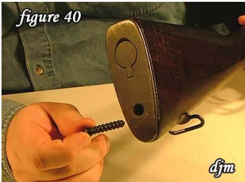
40) Remove the lower butt plate screw.
