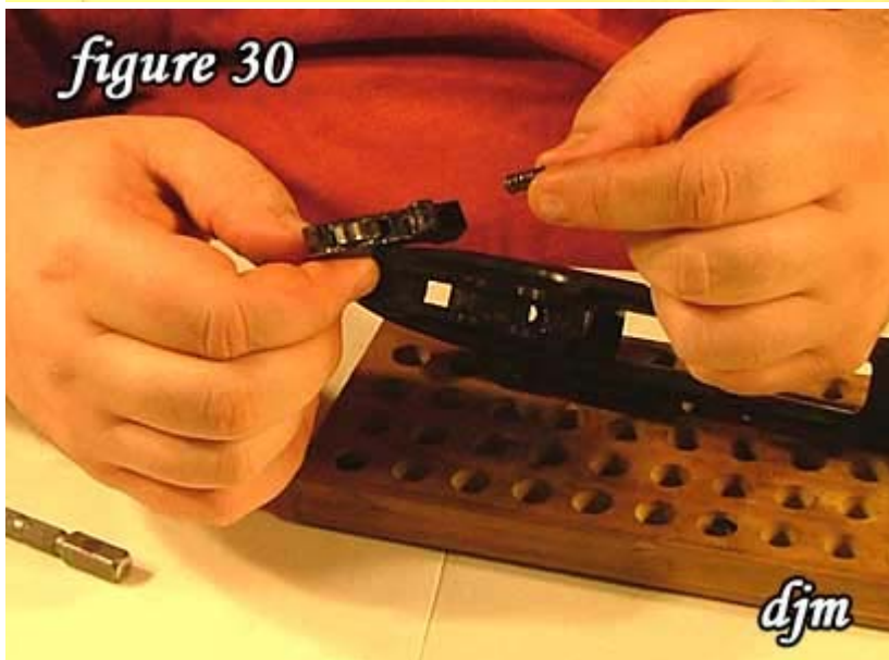
30) Separate the sear spring from the sear.
