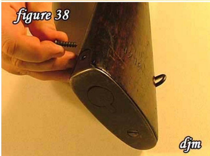
38) Remove the upper butt plate screw.
