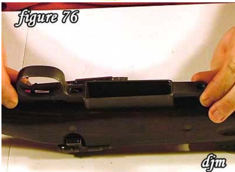
76) Insert the trigger guard into the rifle.
