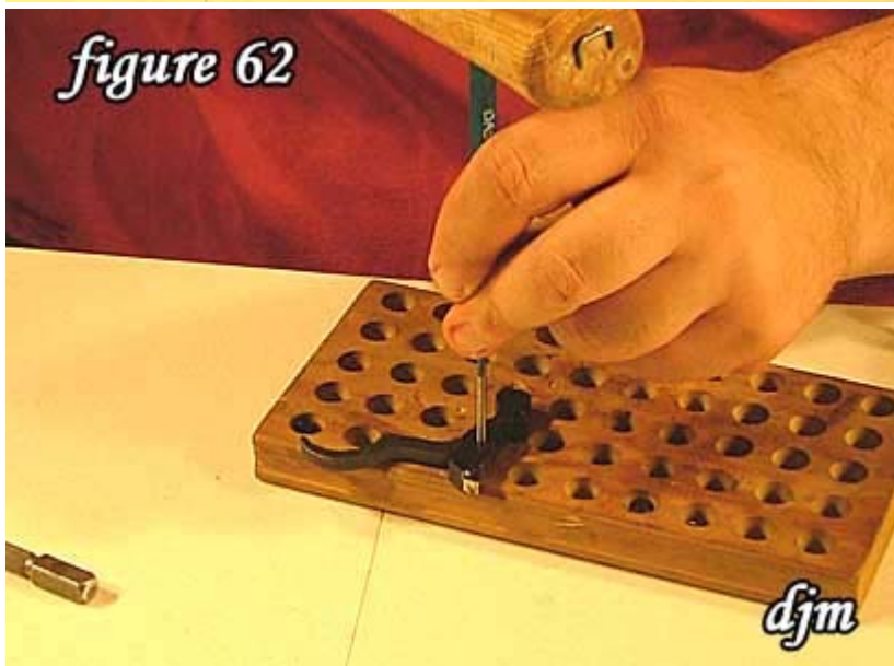
62) Tap trigger pin into place.
