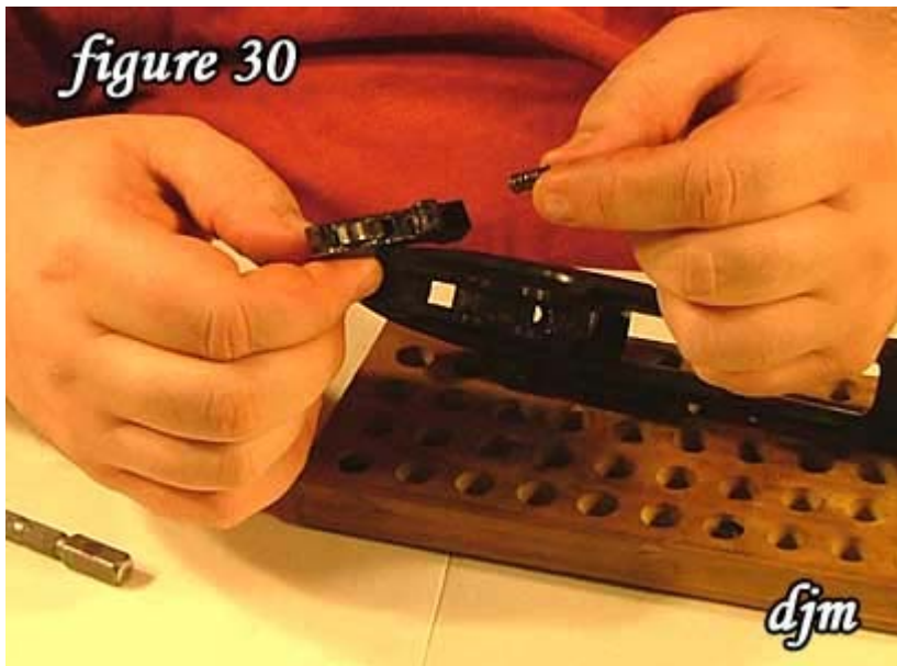
30) Separate the sear spring from the sear.
