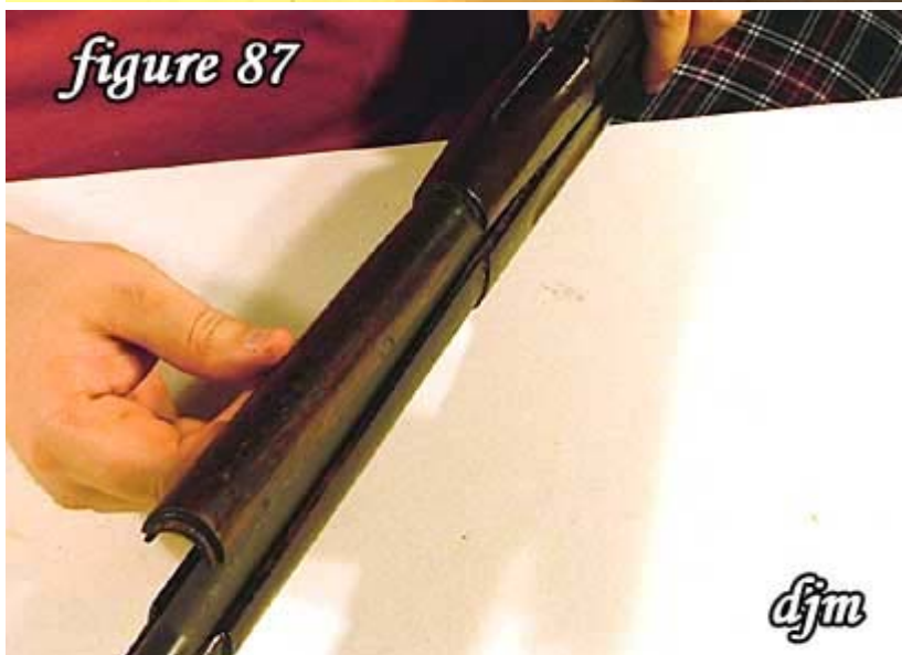
87) Slide the hand guard to the rear of the barrel. If a 03A3 or 03A4 rifle seat hand guard into hang guard ring.
