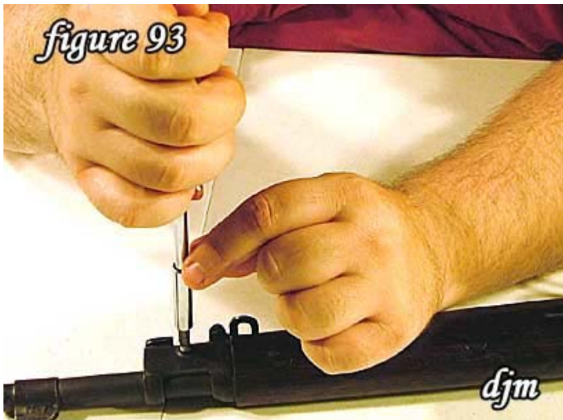
93) Tighten the upper band screw.
