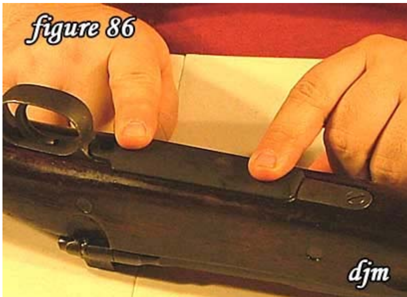
86) (1903 and 1903A1) Snap floor plate in place.
