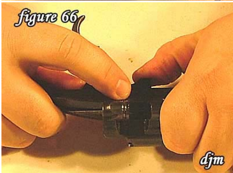
66) Push sear pin all the way into place.
