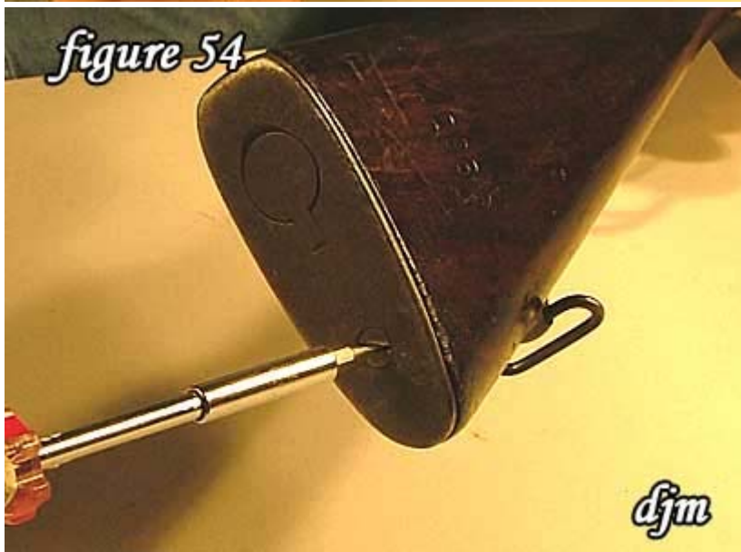
54) Tighten the lower butt plate screw.
