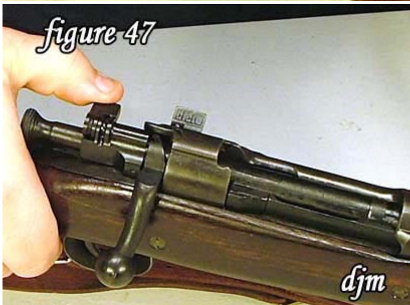
47) Rotate safety lever to "ready" position.
