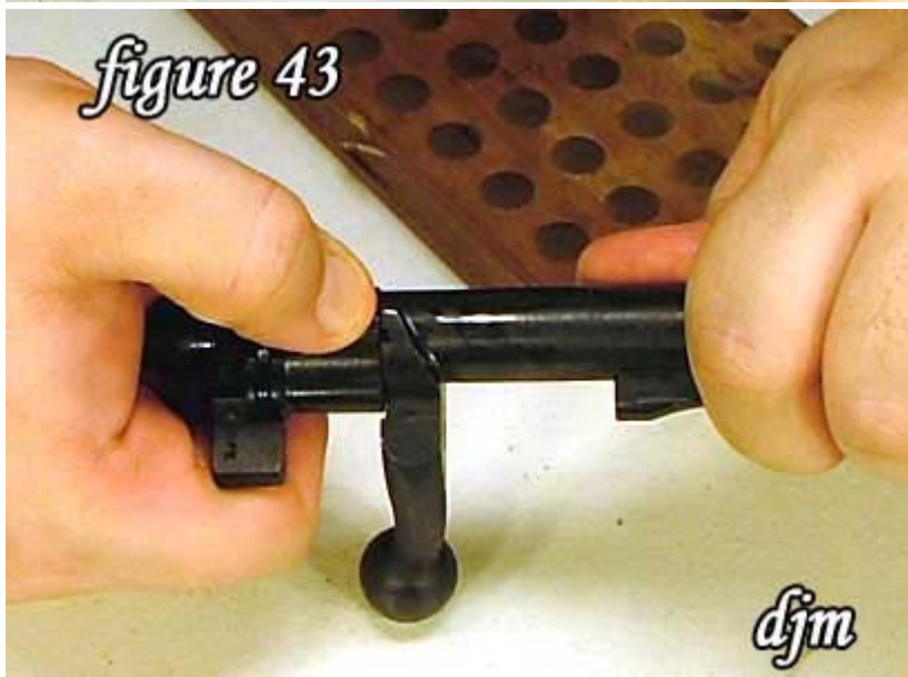
43) Depress bolt sleeve lock and rotate the bolt sleeve into its locked position.
