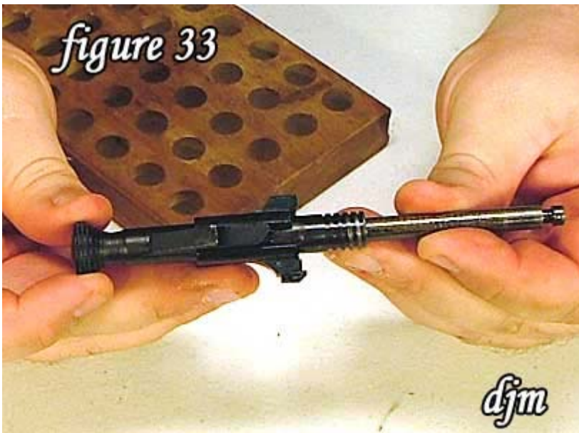
33) Figure 33 shows the position of the sear notch/lug as it rest in the bolt sleeve.
