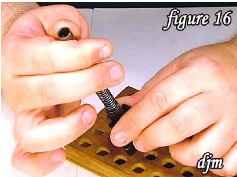
16) Allow the main spring to expand slowly.
