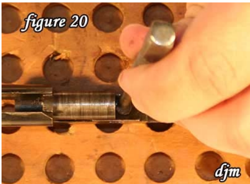
20) Tap the pin into place.
