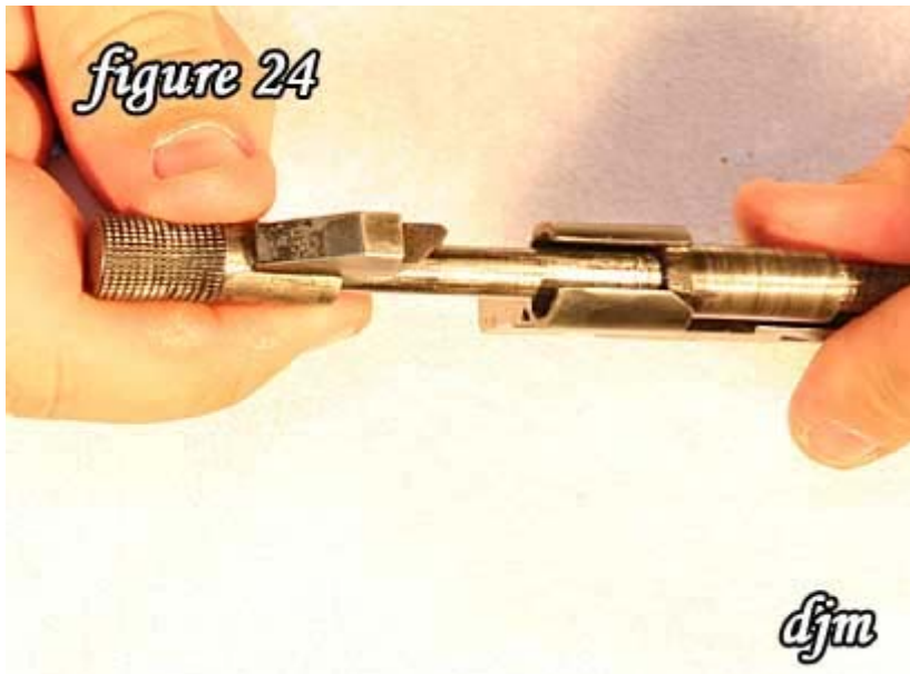
24) Insert firing pin into rear of sleeve.
