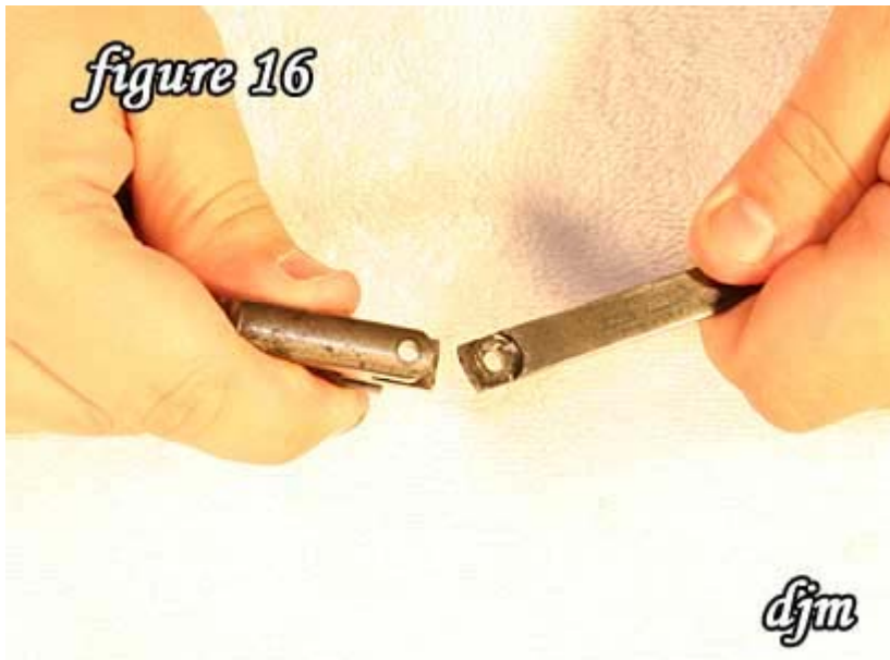
16) Separate the extractor from the sleeve.
