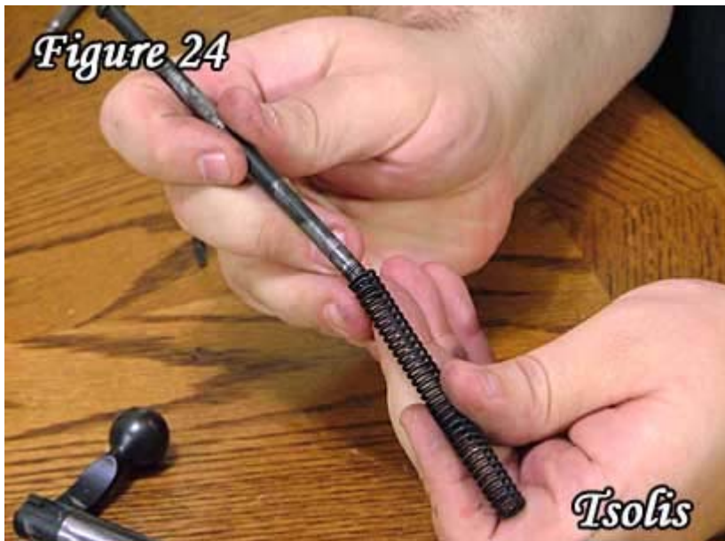
24) Slide the main spring over the rear of the striker.
