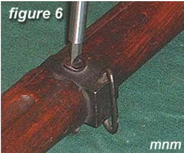
6) Remove the screw on the rear barrel band.
