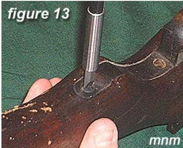
13) Remove the rear trigger guard screw .
