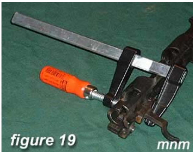
19) I learned a trick to keep the trigger assembly in place while reinstalling the cross pin , as shown in figure 19 .
