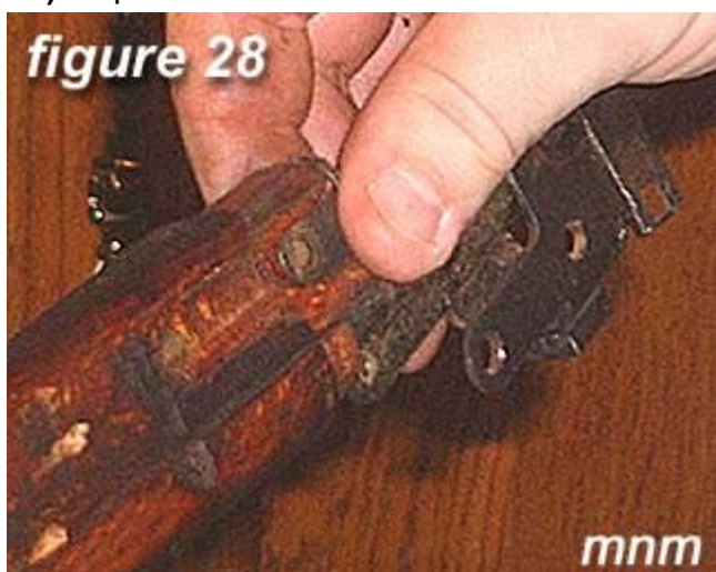
28) Slide forward barrel band back over rifle stock.
