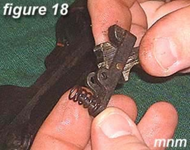
18) Figure 18 shows the trigger assembly with the spring correctly installed.
