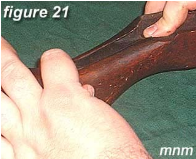
21) Place receiver tang into stock as shown in figure 21 .
