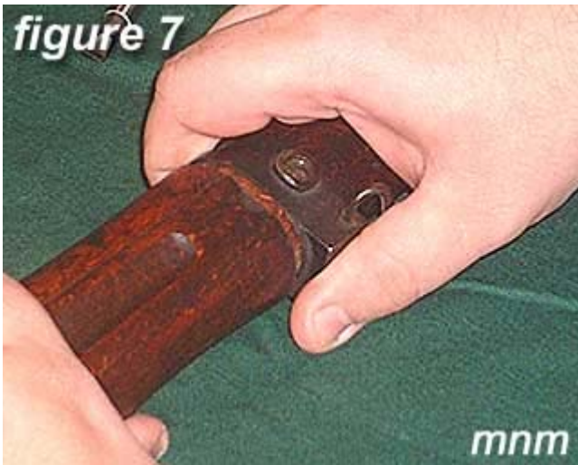
7) Slide the rear barrel band forward.
