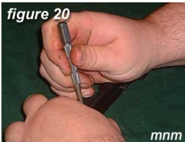
20) Insert cross pin into the trigger assembly with punch.
