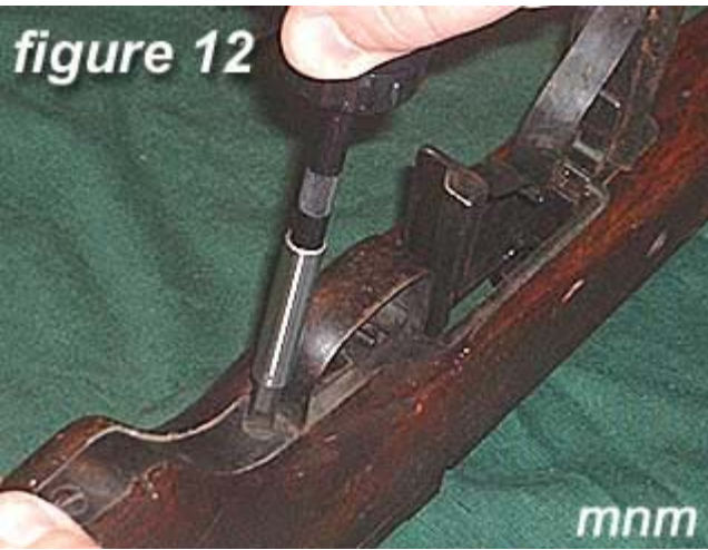
12) Remove the middle trigger guard screw .
