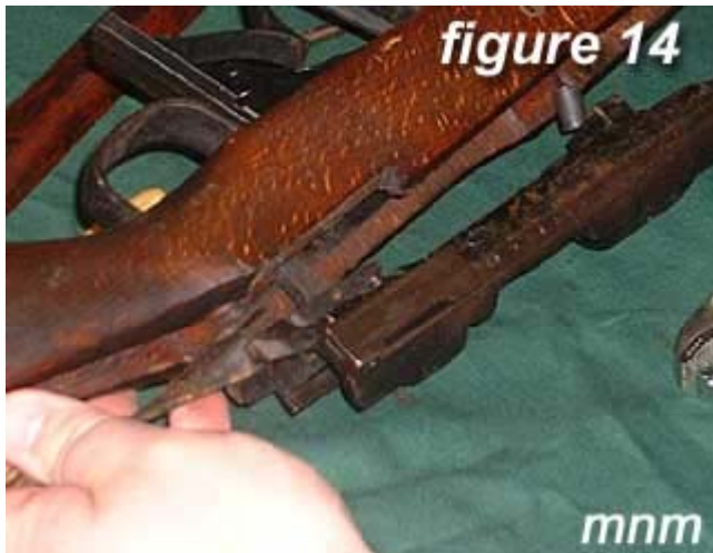
14) Remove the barrel and receiver assembly from the stock . Remove the separate receiver tang also and set aside.
