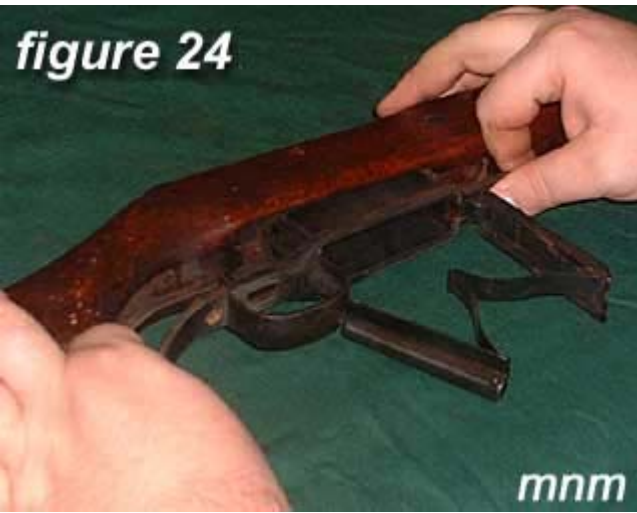
24) Replace magazine cover and install screws .
