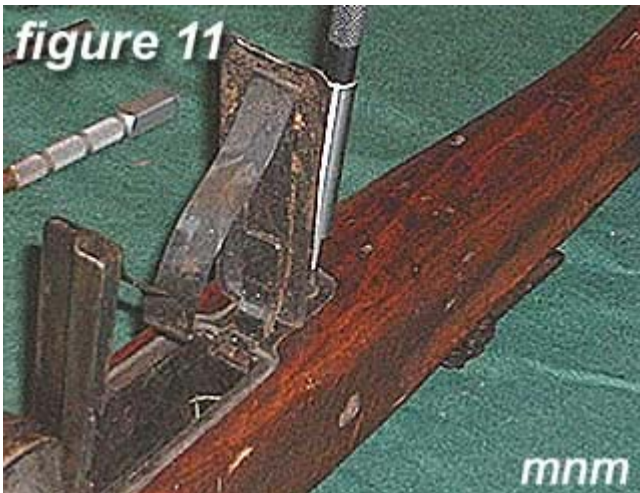
11) Remove the forward trigger guard screw .
