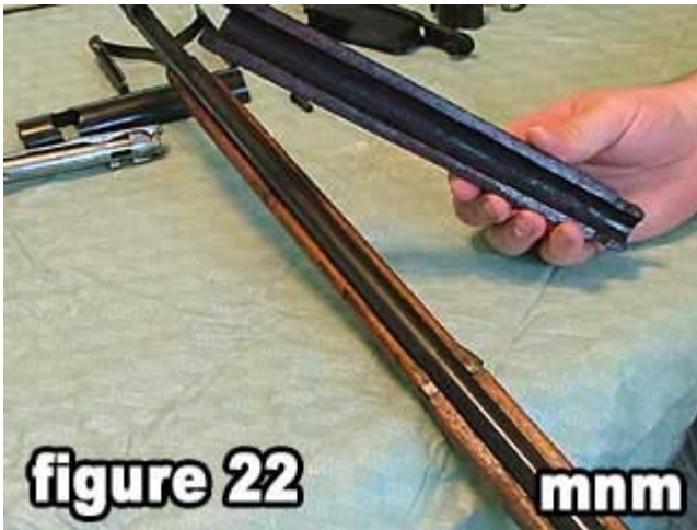
22) Remove the handguard and set aside.
