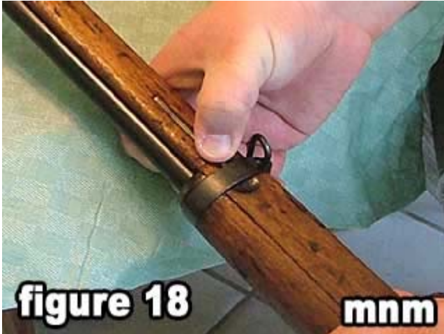
18) Depress the lower band spring .
