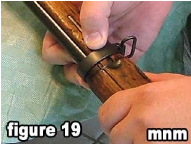
19) While depressing the spring slide the lower band over it.
