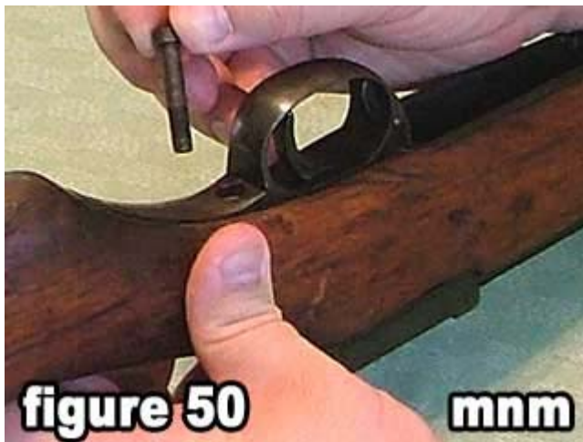
50) Install the rear guard screw.
