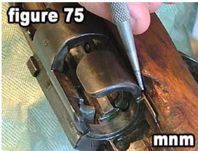
75) Figure 75 shows the right hand receiver cover groove .
