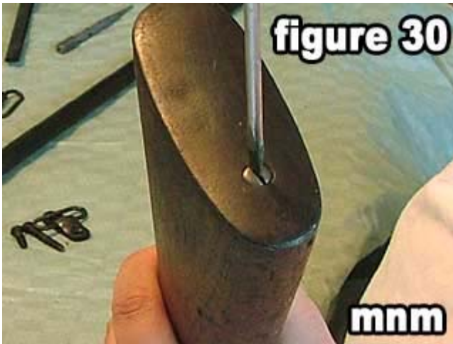
30) Unscrew the lower butt plate screw .
