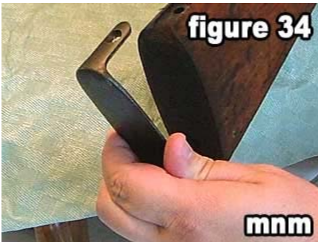
34) Remove the butt plate and set aside.
