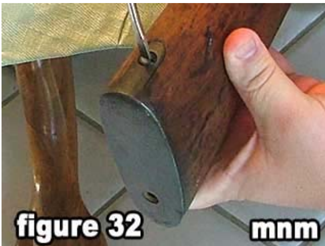
32) Unscrew the upper butt plate screw .
