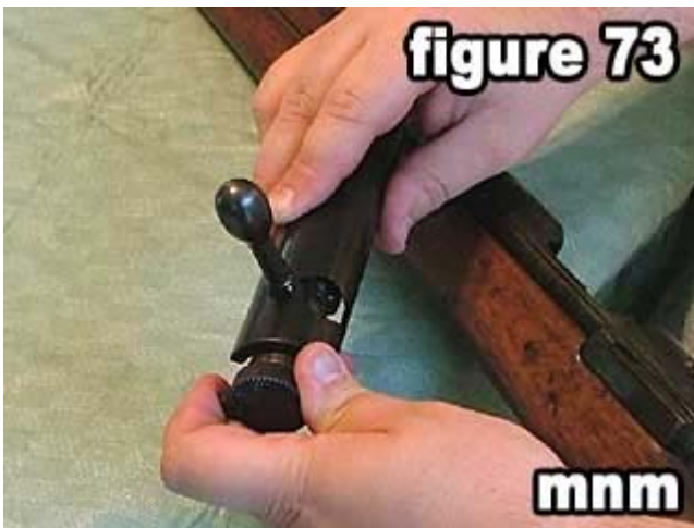
73) Reinstall the bolt/receiver cover back onto the bolt .
