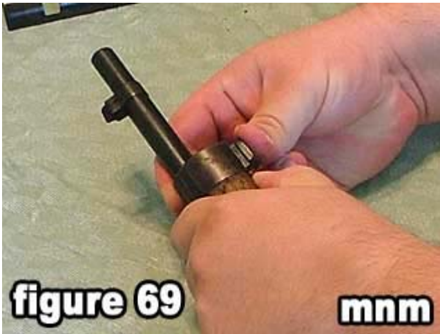
69) Depress the bayonet band spring and slide the bayonet band into place.
