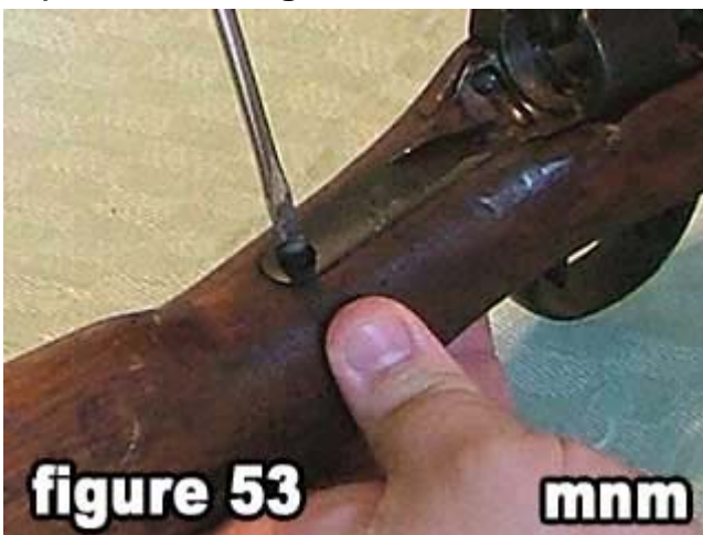
53) Tighten the tang screw.
