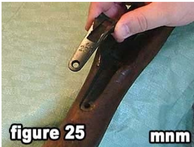
25) Remove the upper tang and set aside.
