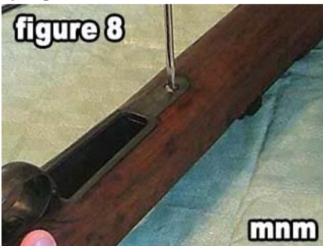
8) Loosen the front guard screw .
