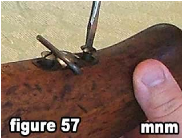
57) Tighten the front swivel screw.
