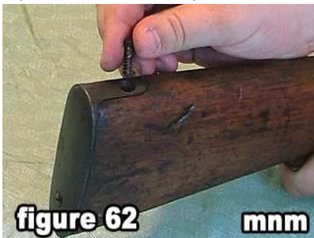
62) Reinstall the upper butt plate screw.
