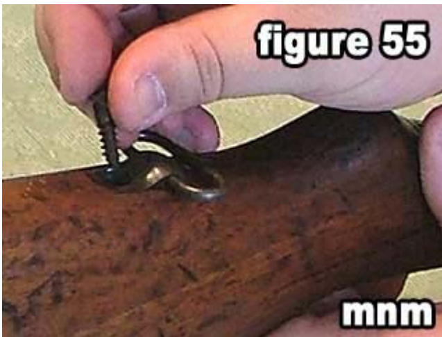
55) Install the rear swivel screw.
