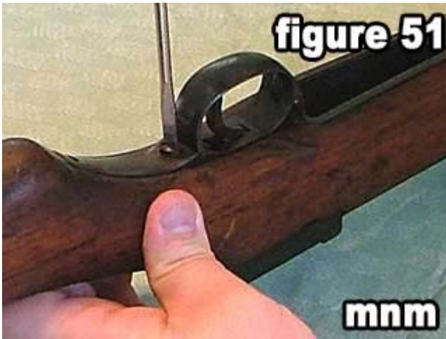
51) Tighten the rear guard screw.
