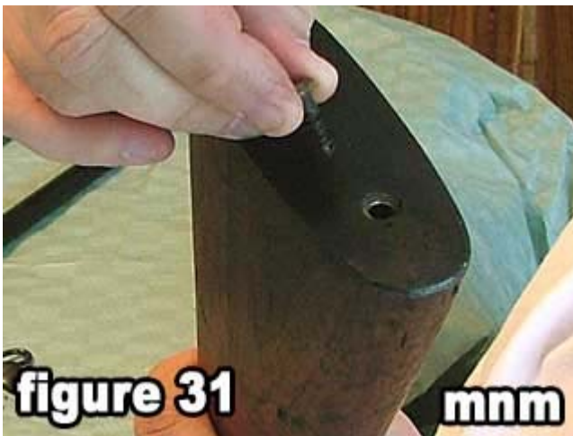
31) Remove the lower butt plate screw .
