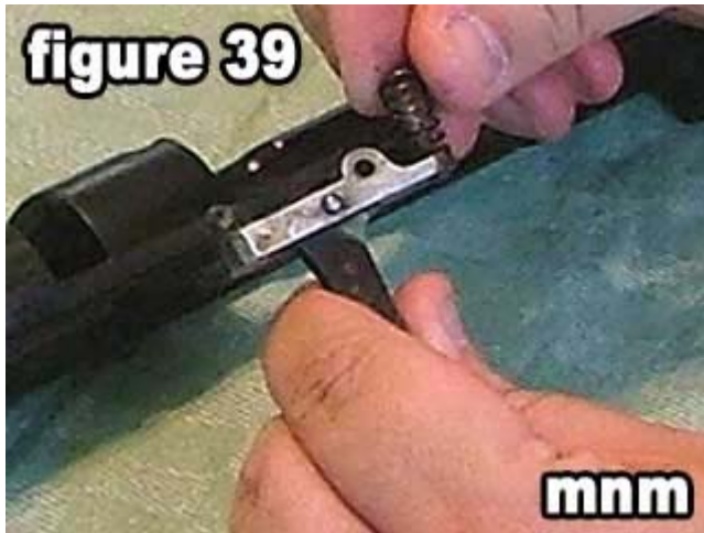
39) Place the sear spring on the sear spring pin on the sear as shown in figure 39 .
