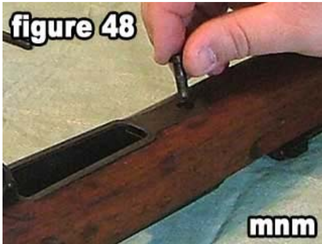
48) Insert the front guard screw.
