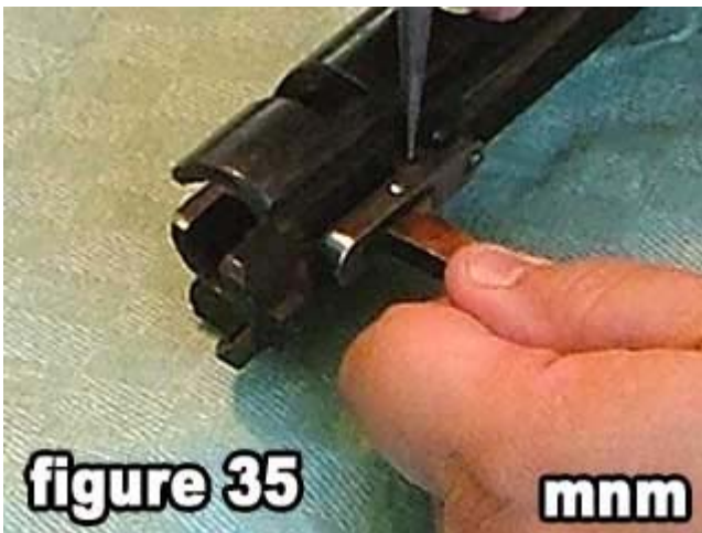
35) Figure 35 shows the sear pin .
