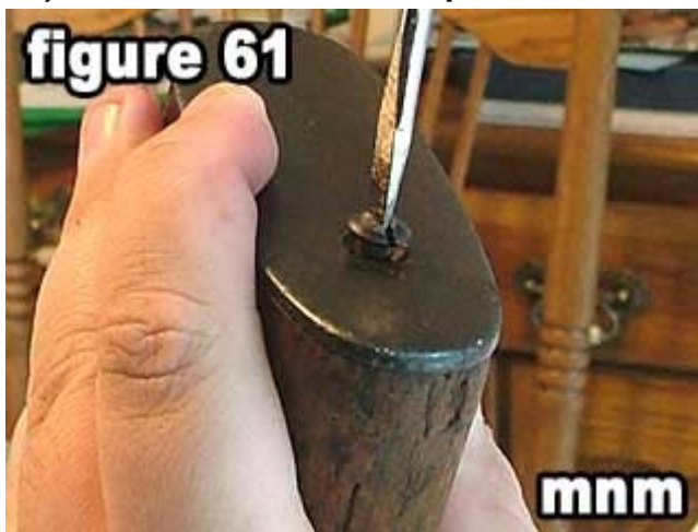
61) Tighten the lower butt plate screw.
