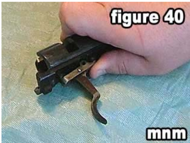
40) Place trigger and sear back onto receiver .
