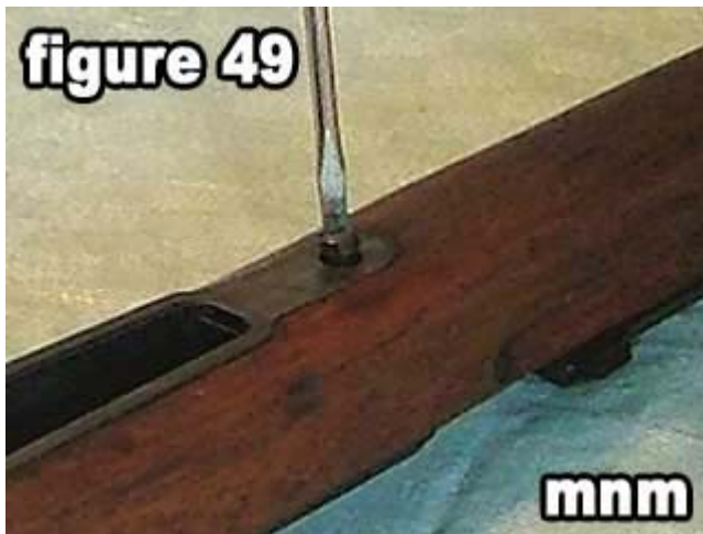
49) Tighten the front guard screw.
