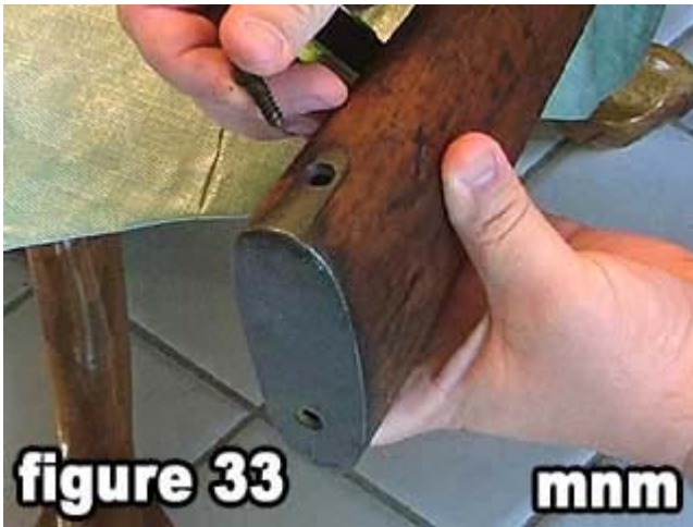
33) Remove the upper butt plate screw .
