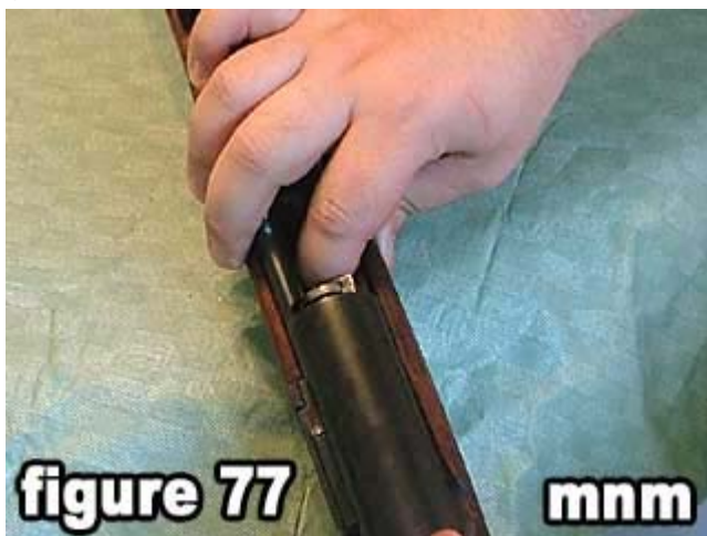
77) Press down on the follower and push the bolt forward.
