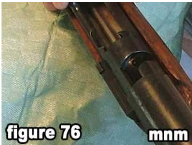
76) Insert the bolt and bolt/receiver cover into the grooves.
