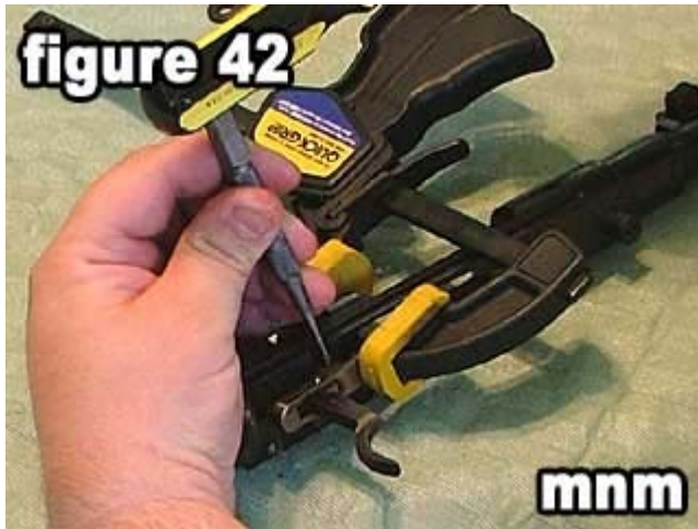
42) Lightly tap the sear pin into the sear .
