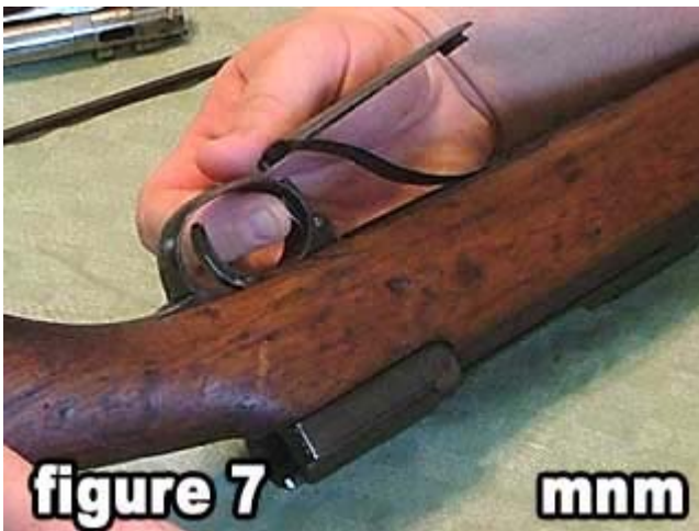
7) Remove the floor plate, follower, and follower spring and set the assembly aside.
