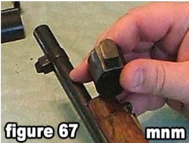
67) Figure 67 shows the direction that the bayonet lug should point in relation to the muzzle.
