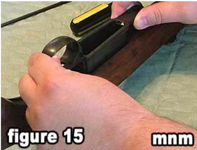
15) Remove the trigger guard/magazine assembly from the stock by pulling it straight up.
