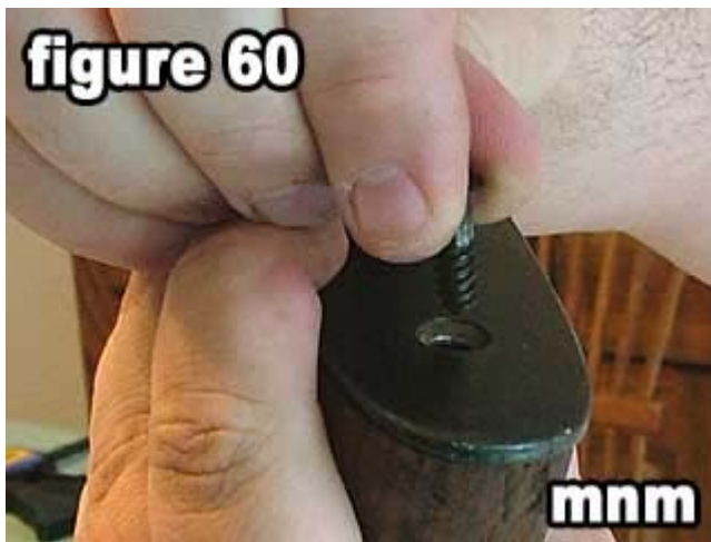
60) Reinstall the lower butt plate screw.
