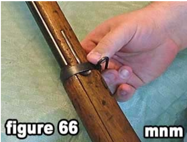
66) While depressing the lower band spring slide the lower band into place.
