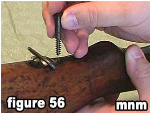
56) Install the front swivel screw.
