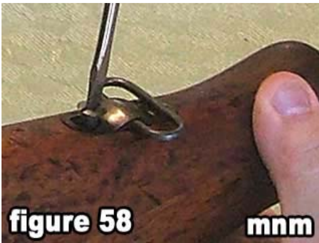
58) Tighten the rear swivel screw.
