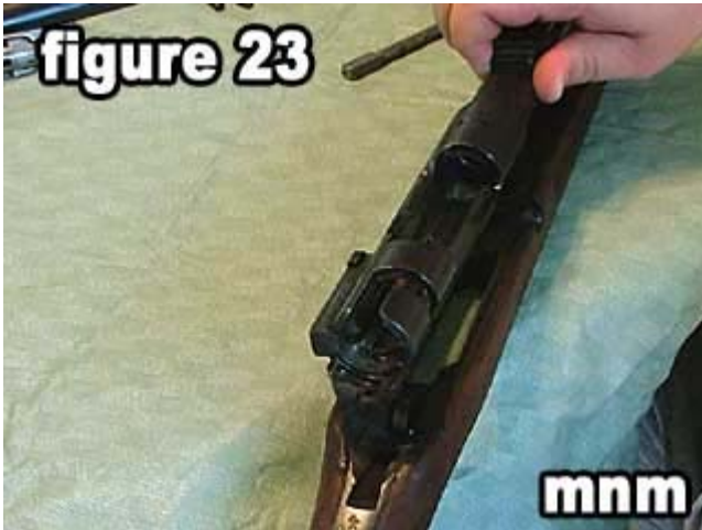
23) Lift out the barreled receiver and set aside.
