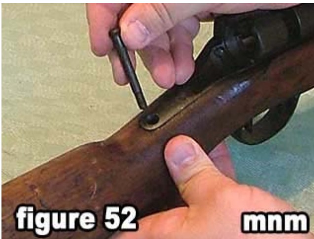
52) Install the tang screw.
