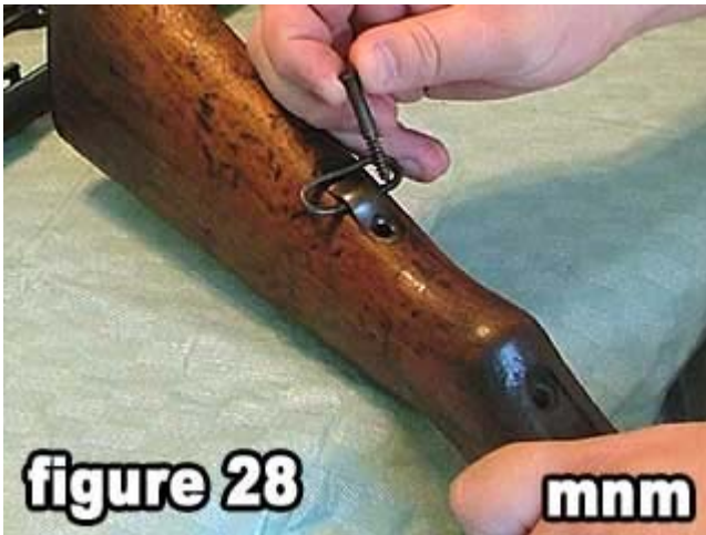
28) Remove the front swivel screw . Note screw length.
