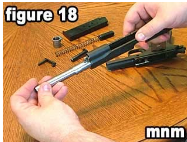
18) Pull the barrel assembly out of the front of the slide and set aside.
