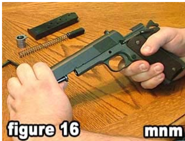
16) Slide the slide forward and off of the receiver frame .
