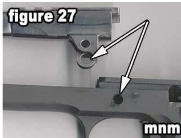
27) Figure 27 shows the slide stop hole and the barrel linkage hole .
