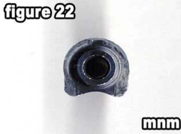
22) Figure 22 shows the rear of the recoil spring guide . Note the inward curved bottom. This rests part against the barrel .
