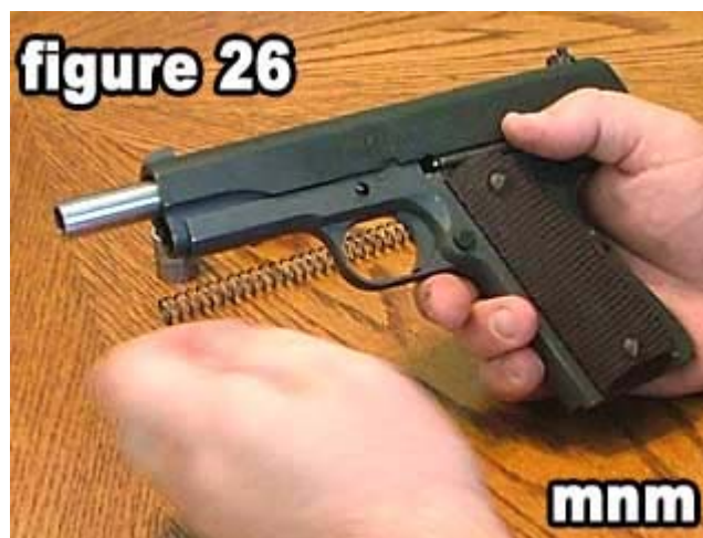
26) Pull the slide back until the rear, small, circular notch in the slide aligns with the rear slide hole .
