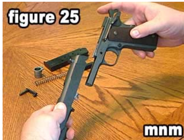
25) While holding the recoil spring guide in place, place the slide onto the frame's rails .
