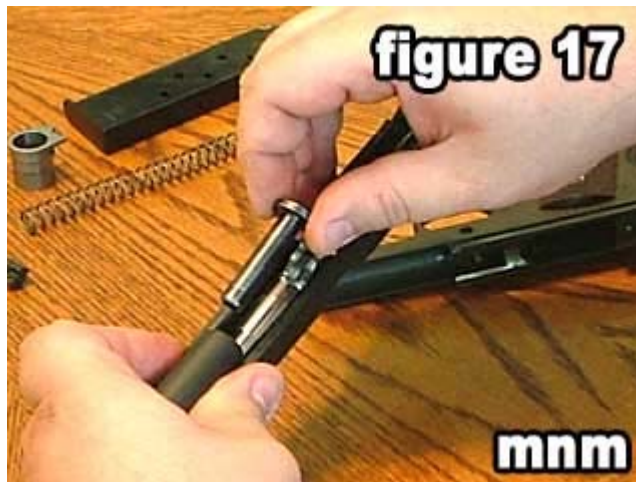
17) Remove the recoil spring guide and set aside.
