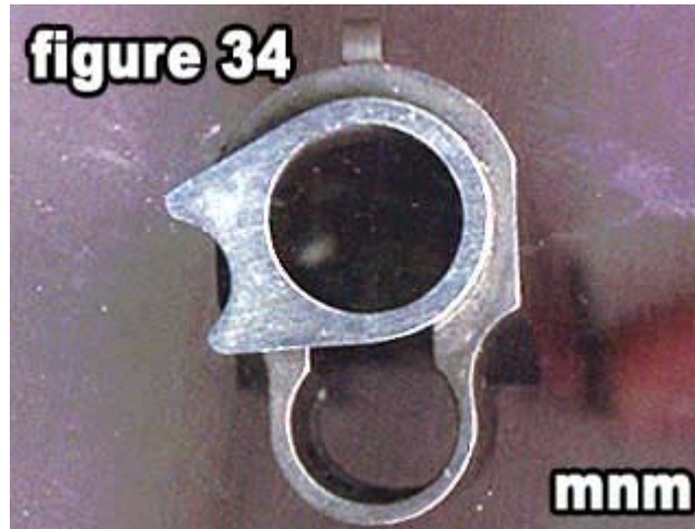
34) Figure 34 shows the position the barrel bushing needs to be in for you to be able to insert the recoil spring and recoil spring plug .
