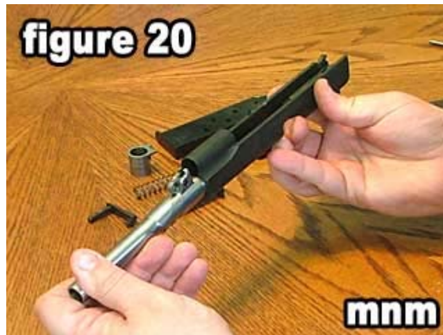
20) Slide the barrel assembly into the slide as shown in figure 20.
