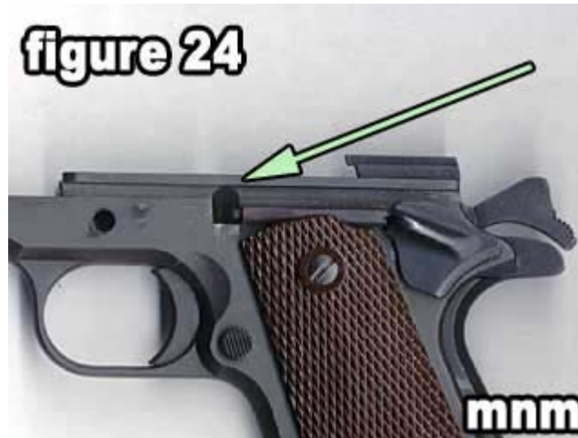
24) Note the arrow pointing to the rails on the side of the frame . The rails are what the slide rides upon.
