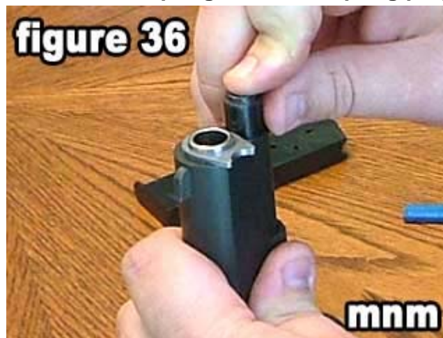
36) Compress the recoil spring and recoil spring plug .
