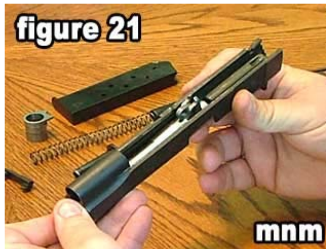
21) Slide the barrel assembly all the way to the rear.
