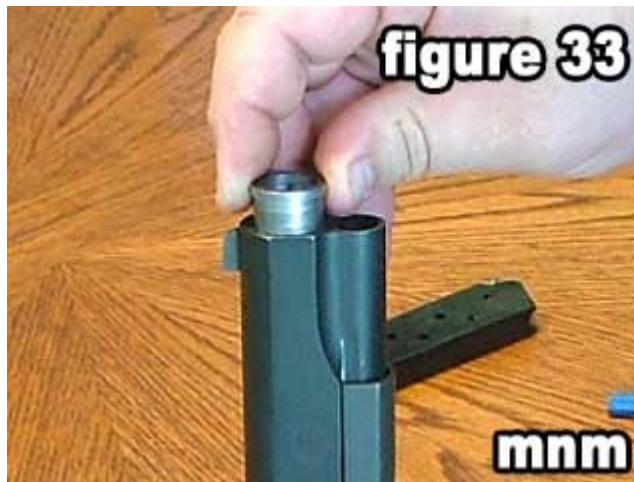
33) Insert the barrel bushing and rotate clockwise all the way.
