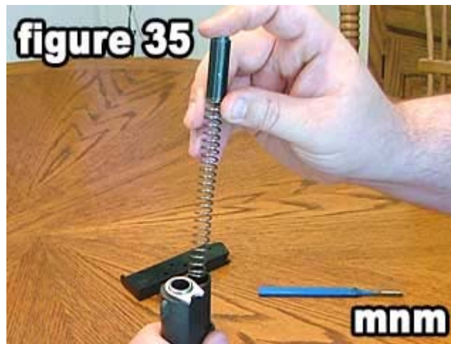
35) Insert the recoil spring and recoil spring plug .
