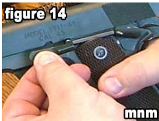
14) Pull the slide stop towards you, removing it from the slide .
